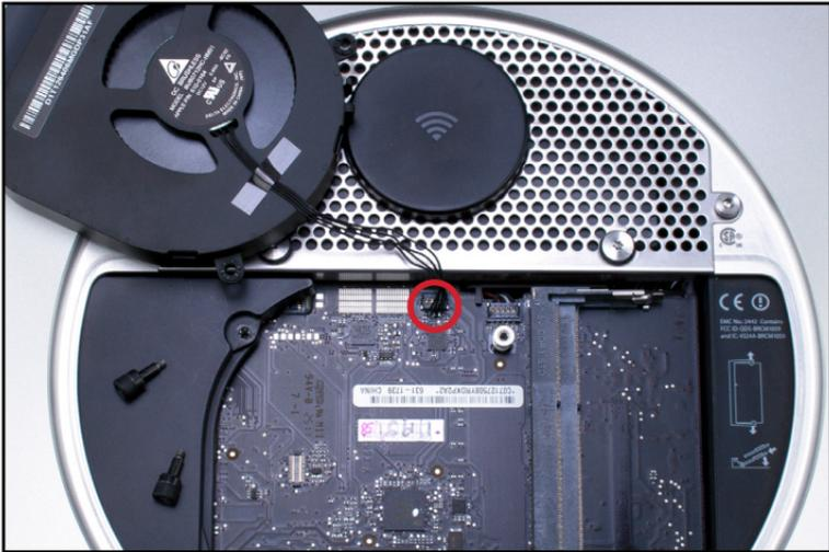
41. Insert and then refasten the three Torx T-6 screws that were removed in **Step 4**; these secure the exhaust fan to the chassis. **NOTE:** The lower-right screw is a longer standoff screw. The other screws are shorter; the longer screw needs to be refastened in its original location.
