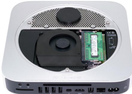
3. Follow the RAM module removal steps that are silk-screened onto the chassis of the Mac mini (highlighted below in red). NOTE: module color may vary.
