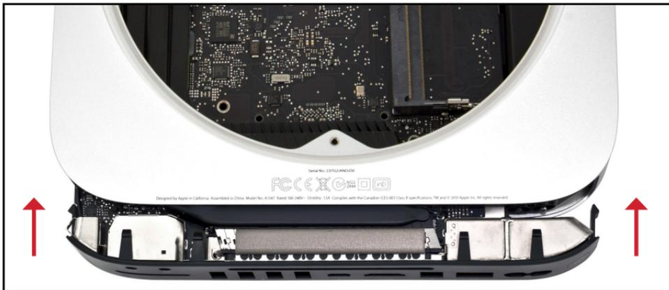
31. Looking from the front of the Mac mini (opposite the side you were looking at in Step 30), locate the power supply plug and carefully reconnect it to the logic board.
