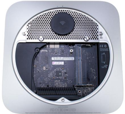
6. Use the Torx T8 driver to remove the three 2mm hex head screws that are used to hold the bottom cover onto the Mac mini (highlighted below in blue). Caution: Do not exert heavy force; the screws are easily stripped. Next, remove the two Torx T8 screws highlighted in red, these screws secure the drive in the lower drive bay.
