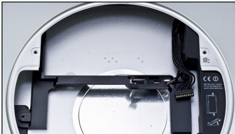
18. Look at the back of the Mac mini and locate the power port. Inside the chassis to the left of the power port is a metal tab that is angled at 45°. Slide this silver metal tab to the left and remove it from the Mac mini chassis, unlocking the power connector.
