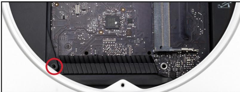
37. Pivot the Airport antenna cover gently into the Mac mini as shown below. Turn the black Airport cable so that the silver connector loops around from the inside-top and attach the connector onto the Airport card. The connector snaps straight down onto the card. **CAUTION:** the antenna and cable are easily damaged.
