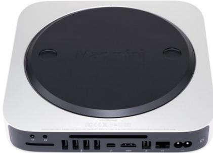
2. Remove the bottom cover of the Mac mini to expose its internal components.
