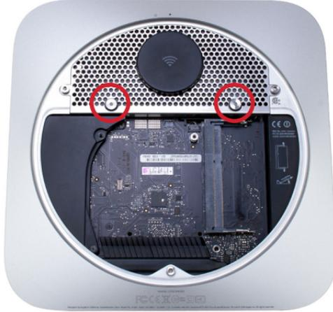
7. Gently lift the Airport antenna cover from the side closest to the logic board, as shown below-left. Next, slide the Airport antenna cover towards you and rotate it about 45 degrees as shown below-right. The antenna connector is under a hinged black plastic cover. Gently lift the cover to expose the connector as shown at top-right, then very carefully lift the connector to remove it from the Mac mini. **CAUTION:** this cable assembly is easily damaged.
