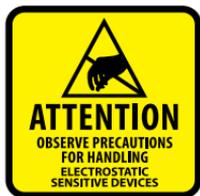
Your computer is a static-sensitive device. It is susceptible to invisible damage if not protected during installation. We recommend proper grounding through use of a grounding strap. Always work in a clean and static-free area, and avoid wearing clothing that retains static charges. For more information, please visit: [www.owcdigital.com/support/anti-static](http://www.owcdigital.com/support/anti-static)
