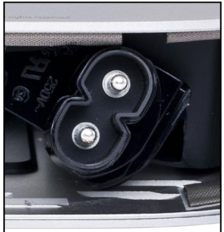
20. Slide the power supply out of the Mac mini chassis. You may have to lift the mounting tab (highlighted below in red) before the power supply will slide smoothly.
