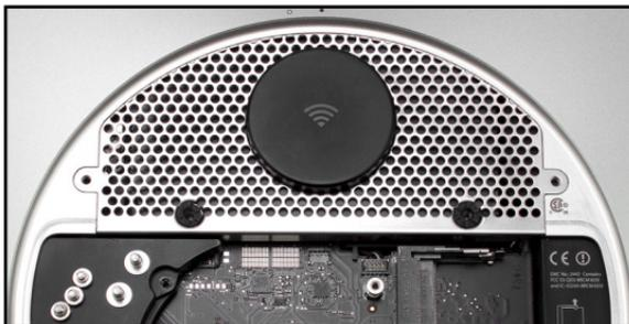
39. Using the Torx T8 driver, insert the five screws that you removed in **Step 6**. Make sure the hex head screws (highlighted in blue) and Torx screws (highlighted in red) are placed back in their original locations. Use a Torx T8 driver to secure all five screws. **CAUTION:** do not to over-tighten the screws; they are easily stripped.
