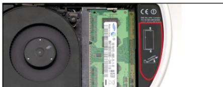
4. Remove the three Torx T-6 screws that secure the exhaust fan to the Mac mini chassis. NOTE: The lower-right screw is a longer standoff screw. The other screws are shorter; all three need to be refastened in the same locations later.
