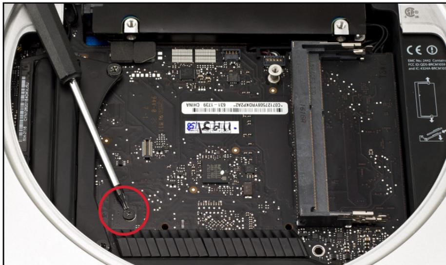
35. Reseat the fan cowling that you removed in Step 9, as shown below.
