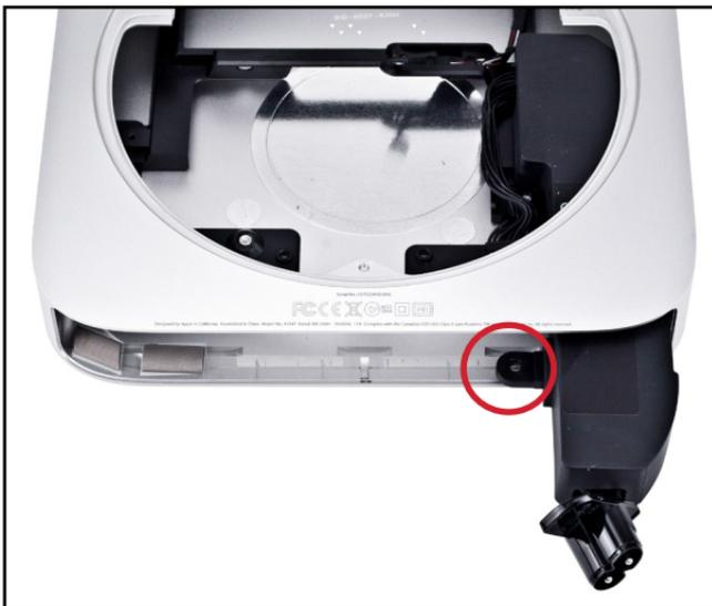
21. Lift up on the hard drive carrier and remove it from the Mac mini chassis.
