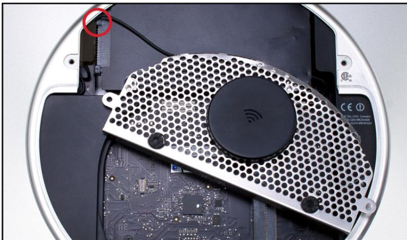
38. Carefully align the Airport antenna cover and slide it into place as shown below. The edge of the cover will slip into a channel cut out in the chassis. Make sure it is straight and seated level before continuing. NOTE: if you are unable to get the antenna cover to sit flush, you will have work backwards and attempt to reseal the drive that you installed in **Step 32**, then work back to this step to reseal the antenna cover.
