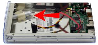
Remove the taped down packet of screws.
