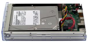
Insert the power and SATA cables into the back of the hard drive and place the drive mechanism into the enclosure.
