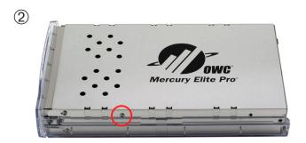
Then, remove the single Phillips screw securing the top metal shield. Lift up on it to remove, exposing the inside of the enclosure.
