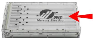
Place the top cover back onto the OWC Mercury Elite Pro, sliding it into the guide rails.
