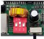
Once you remove the back of the OWC Mercury Elite Pro Dual mini, you will be able to see the red DIP Switch block at the rear of the bridge card, next to the power switch. You need to adjust the DIP switches to change the RAID mode. **Note that ON is UP, or towards the INSIDE of the enclosure.**
