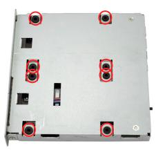
With your fingers holding the drive mechanisms into the enclosure, flip it over onto the top so you can see the screw holes that you will need to use in the next step.
