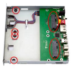
Once the inner chassis is removed from the outer shell, you will see where your 2.5" SATA drives will attach to the bridge card.
