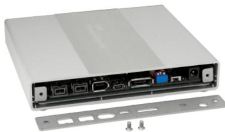
⑧ Once you have installed the drive mechanisms, simply slide the inner chassis back through the outer shell. The outer shell can be installed in either direction, but there is a notch on one side that allows the back plate to fit properly. If your case gets turned around and the back plate does not fit correctly, try reinstalling it from the other side.
