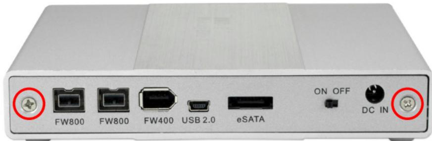
Using a Phillips P0 screwdriver, remove the 2 screws that hold the rear backplane cover to the enclosure.
