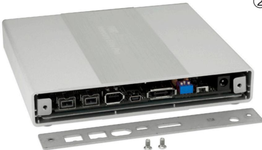
Once the screws are removed, the rear backplane cover will easily come off.
