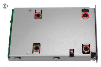
With your fingers holding the drive mechanism into the enclosure, turn it over so you can see the screw holes that you will need to use in the next step.
