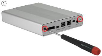
Use a Phillips P0 screwdriver to remove the 2 screws holding the rear backplane cover in place.
