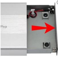
From the rear of the enclosure, press inwards on the rear ports to slide the inner chassis out towards the front of the enclosure.
