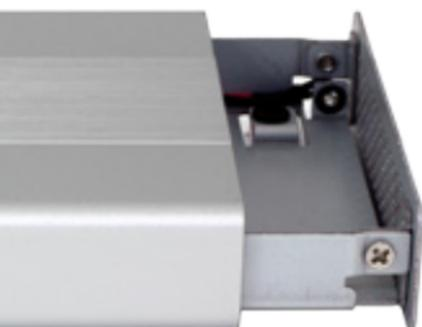
3. Gently push on the inner chassis that was exposed by removing the back plate. The inner chassis should slide out of the outer enclosure. Once there is enough room at the front, as shown to the left, you can pull on the front of the inner chassis to remove it fully.
