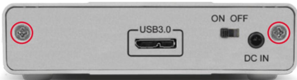
2. Tilt the Mercury Elite Pro mini up at the front to allow the back plate to fall free, as shown below. If the back plate does not immediately fall free, you can push gently on the on/off switch to disengage the ports from the back plate and allow it to come off.
