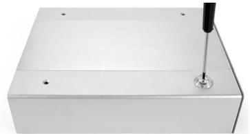
3. Push on the rear cover plate in order to slide the inner chassis out of the outer enclosure, as shown at right. Do not grasp the inner chassis by the front bezel, as it may bend slightly. Remove the screw packet and set it aside.
