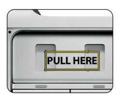
3. Grasp the optical drive carrier and pull it straight out. Disconnect the power and data cables from the back of the existing optical drive and set the carrier in front of you.
