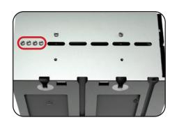
4. Insert your new SATA optical drive into the carrier, in the empty lower bay. There should be four screws provided by Apple, inserted on the back side of the carrier (highlighted at left). Remove them and use them to fasten the new optical drive drive to the carrier (two on each side).
