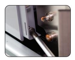
12. (2007 Mac Pro only) There is a hidden Phillips screw located at the base of the fan assembly (left). Remove it. Take care not to drop the screw once it is loose. We recommend a magnetic-tipped screwdriver for this step as well.
