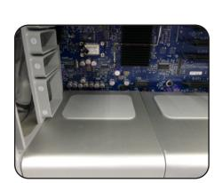
2007 Mac Pro - lift the back of the CPU heat sink cover upward, then outward towards you (below-left). It is held in place by magnets and should come loose easily.
