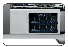
(2006 model only) Locate the memory bay (shown left). Grip the upper memory board by the circular cut-outs (shown below-left), then pull the board straight out of its slot and set it aside. Repeat the process with the lower memory board.
