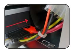
9. Carefully guide the drive carrier back into the optical drive bay. There are two screws that slot into cutouts on the carrier. Carefully route the cables so that they are not pinched or disconnected when fitting the carrier into the optical bay. If you feel any resistance, remove the carrier and look for wires or cables that may be in the way. Do not push through the resistance or you could damage the wires or cables.
