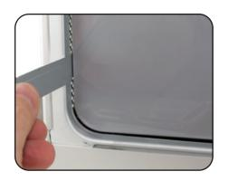
13. Take the PCle cover you removed in Step 7. Starting at the top of the fan assembly, work the short end of the bracket into the gap at the front of the Mac Pro, shown at left.
