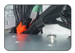
5. Start routing the SATA cable that you have attached to the logic board in Step 2 up through the corner of the optical bay, following the existing wires that are shown below.
