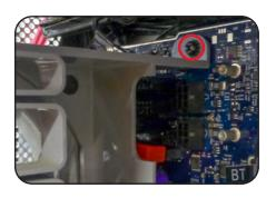
7. Reinsert the fan assembly into the computer, sliding it on its base track and then re-affixing the Phillips screw that was removed earlier (shown at left). Make sure that the cable is not pinned behind the fan assembly when you tighten the screw.
