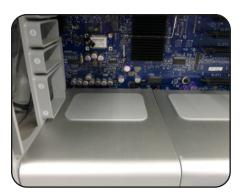
4. Lift the back of the CPU heat sink cover upward, then outward towards you (below-left). It is held in place by magnets and should come loose easily.
