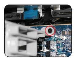
3. To the left of the PCle slots, at the top of the logic board, remove the Phillips screw (highlighted at left) using a Phillips P0 driver. We recommend a magnetic-tipped driver.
