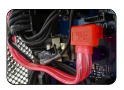
You may have to experiment to get the proper routing, based on the configuration of your Mac Pro. Make sure the cable is positioned so that it will not get crimped or pinned against other connectors on the logic board.
