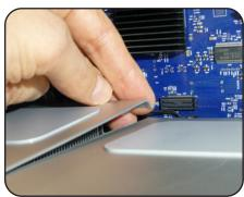
5. Loosen and remove the silver colored Phillips screw from the bottom-right edge of the fan assembly. Take care not to drop the screw once it is loose. We recommend a magnetic-tipped screwdriver for this step as well.
