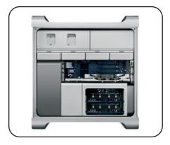
Disconnect power and all other device cables from the Mac Pro. Lift the latch on the back of the case then remove the side cover and set it aside.
