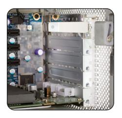
7. Once the retaining plate is removed, remove the PCle cover from the top slot, shown at left. Set it aside; you will need it again at Step 13.
