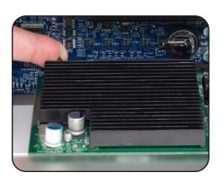
8. Next, find the GPU and note its connection to the PCle slot. There is a small plastic tab at the left end of the slot — lift it upward as shown. While doing this, pull the card toward you to remove it from the PCle slot. Set the GPU aside.
