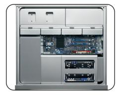
1. Disconnect power and all other device cables from the Mac Pro. Lift the latch on the back of the Mac Pro then remove the side cover and set it aside.
