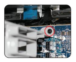
9. To the left of the PCle slots, at the top of the logic board, carefully remove the Phillips screw (shown at left) using a Phillips P0 driver. We recommend a magnetic-tipped driver.
