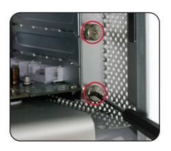
6. Using your fingers or a Phillips driver, loosen the thumbscrews that hold the PCle cover retaining plate in place, then remove it. NOTE: there is a tab at the top of the retaining plate that helps to hold it in place — once the thumbscrews are loosened, slide the plate downward before pulling it out of the case.
