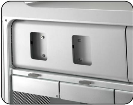
10. Once the cables are attached, fully seat the optical drive cage back into the Mac Pro chassis. Reseat and secure the side panel that was removed in Step 1 to complete the process.
