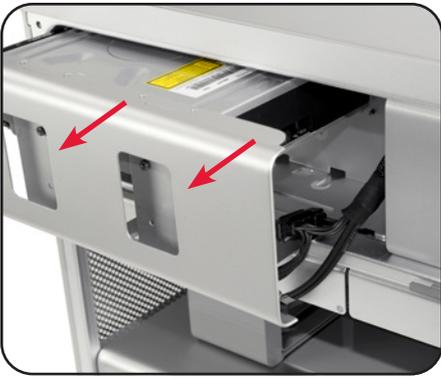
1. Shut down the Mac Pro and remove the side panel. Pull the optical bay drive cage using the recessed handles (shown at left) and slide it out of the optical bay until you can see the two black cables attached to the optical drive. Disconnect the cables, then fully remove the cage and set it on a work surface.
