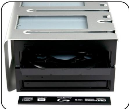
8. The photo at left shows the bezel removed. At this point you can slide the drive tray back into the drive until it locks back into place.
