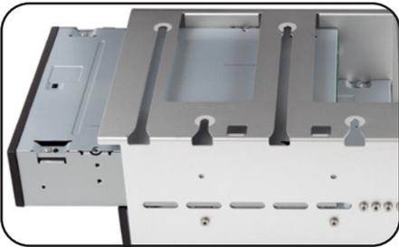
3. Slide the new optical drive into the optical bay, ports first, until the front bezel lines up with the factory optical drive. The image at left shows the bottom of the drive cage and optical drive being slotted into place.
