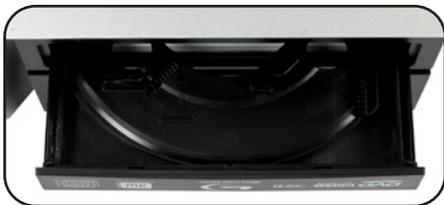
7. Turn the assembly over so you have the vantage point shown at left. Here the bezel to be removed has white logos on it. Gently pry the bezel towards you and it should pop off.
