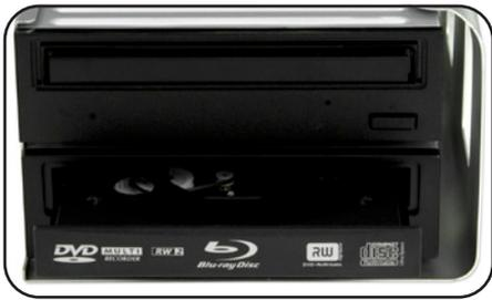
6. Insert a straightened paper clip into the manual disc eject hole on the front of the optical drive; apply moderate pressure until the drive tray slides out. Carefully pull the tray out about two inches.
