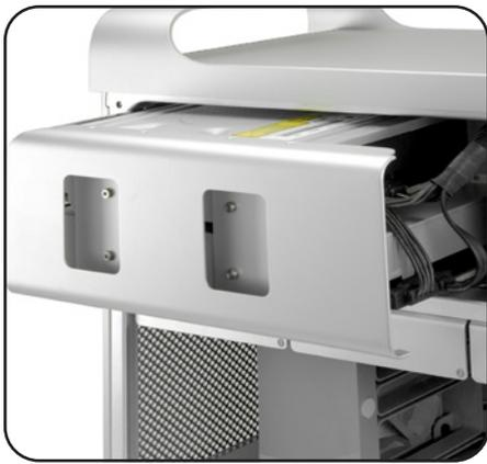
9. Slide the drive cage back into the Mac Pro's optical bay, making sure to align the slots on the bottom of the cage so that they slide over the metal posts on the bottom of the bay. Be sure to leave enough room to connect the power and SATA cables to the optical drive(s).
