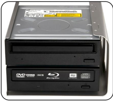
5. Turn the optical bay assembly so you can see the front bezels on the optical drives. Notice there is no drive door on the factory original drive; you need to remove the drive door on the new drive as well to allow it to eject through the sliding door on the front of the Mac Pro.
