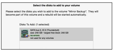
5. The rebuild process will begin automatically as soon as you confirm the addition of the new disk to the RAID volume. Note that the disk tile shows the predicted time remaining to rebuild the volume, as well as a progress meter on the volume icon.
