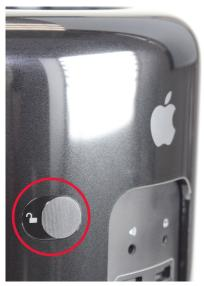
Turn off your Mac Pro and unplug all cables, including the power cable. Make sure the lock switch on the outer case is set to the unlocked position (circled at left), then remove the outer case by lifting it straight up. Set aside the outer case and proceed to the next step.
