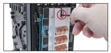
4. Using the included driver, remove the two Torx T8 security screws from the upper right-hand side of the Mac Pro (circled below). **NOTE:** The screws included with this kit are intended only for use with the Aura SSD. If you uninstall the Aura, you must use the original Apple screws to reinstall Apple's SSD; please store them in a safe place.
