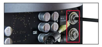
6. Properly installed, the Aura SSD for Mac Pro and power cable will look like the picture below (left). Replace the outer case of the Mac Pro as shown (below right). When the outer case is seated fully, slide the lock switch back to its original locked position.
