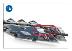
2. Install the SSD into the Mac Pro, as shown below. Insert the SSD at a shallow angle, making sure that the power cable is out of the way.
