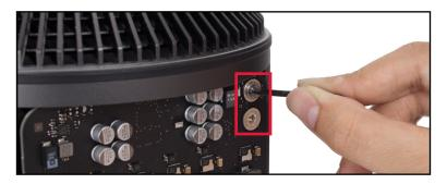
5. First, thread the two included washers onto the two included Torx T8 screws. Next, align the rings on the power cables with the two screw holes, then secure each cable to the power terminals as shown below. Make sure the screws are tightened enough that the power cables cannot rotate in place or move. IMPORTANT: the wire with the black sleeve should always connect to the lower power terminal.
