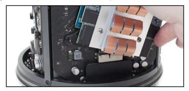
3. Verify that the SSD is fully seated in the connector on the Mac Pro and that the screw hole in the SSD lines up with the screw hole in the Mac Pro. Then, use the included driver and drive mount screw to secure the SSD.
