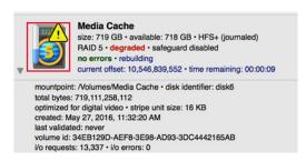
You will be able to use the RAID volume during the rebuild process. Make sure the computer is not powered off or put into sleep mode, and keep the ThunderBay turned on and connected to the computer during this process, or the rebuild will be interrupted.
