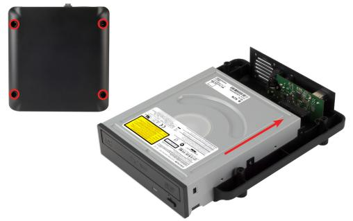
Begin by removing the top cover from your OWC "Value Line" enclosure. Turn the enclosure over and remove the 4 Phillips screws from the bottom and them remove the top cover by lifting it straight off, exposing the interior of the case and green bridge card.
