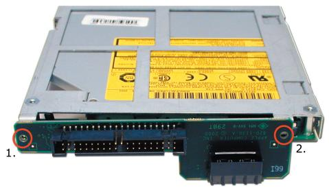
Align the backpanel connector onto the new optical drive as shown and press it's connector into place. You will see that it rocks back and forth a bit on the connector, you will need to insert the included replacement screws to tighten it down properly.
