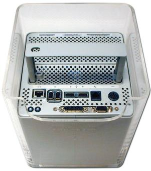
Begin by turning your G4 Cube over on it's top. You will want to place the computer on a soft cloth or a rubber mat to keep it from sliding around while you perform this upgrade. A mouse pad works well, just be sure to not scratch the top of your Cube.
