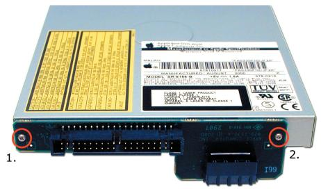
Once the stock optical drive is removed. place it on the table in front of you and look at the backpanel connector. This will need to be removed and transferred to the new drive you're installing.
