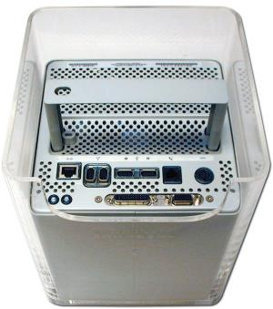
Retrieve the top Cube shell and place it on it's top on a soft surface. Turn the Cube core over and press the locking handle in to release it, and then gently insert the core back into the shell. Press the latch mechanism down to lock it into place, and reattach all of your cables.
