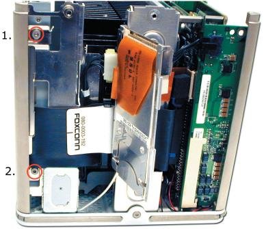
Look at the side of the core that has the Airport card access door on it. If you have an Airport card, you will need to remove it to gain access to this area. The Airport card simply clips in and slides into it's slot, with the antenna plugged into the end. For instructions on how to install or remove the Airport card, refer to your Power Macintosh G4 Cube manual.
