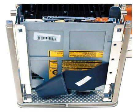
Slide the new optical drive back down into the slot you removed it from, and reattach the IDE and power cords. You may want to do the attachment with the drive lifted up a bit in the slot, it does make for easier access for your fingers.
