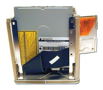
Gently lift upward on the optical drive, it will slide in it's track mount a bit. GENTLY remove the IDE ribon cable from the backpanel connector. The IDE cable will detach downward toward the bottom of the cube.
