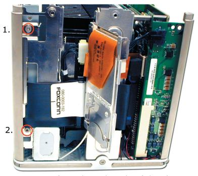
Replace the two Torx T-10 screws from the right side of the chassis. Notice one of the holes is exact sized, and the other is eccentric to allow for adjustment, you won't need to adjust the depth at all, the custom bracketry that the drive uses is perfectly aligned already. Close the Airport access door, and reinsert the Airport card (if equipped).
