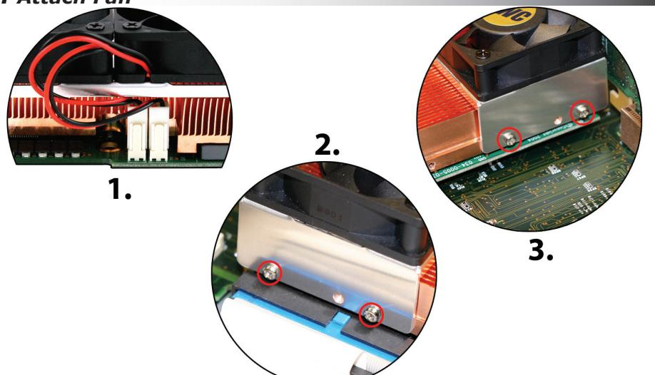
Plug the 2 fan connectors onto the CPU upgrade daughter card. Insert the 4 included small Phillips screws through the holes in the fan assembly and attach to the heatsink in the location shown. You may need to remove the video card to insert the screws more easily. Some systems do not have enough clearance to screw in the screws - 2 will hold the assembly without issue.
