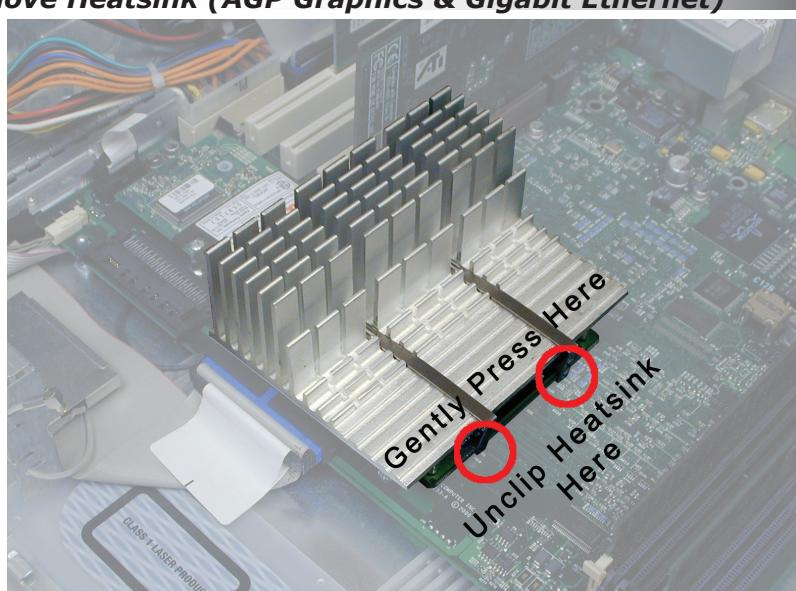
Remove the heatsink from your logic board. Use the needle nose pliers to unhook the clips from the processor card.
