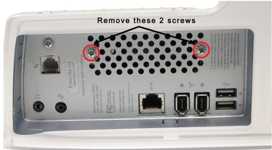
Unscrew these two screws from the rear port panel on your system. This will release the fan from behind the heatsink and allow you to unhook the rear heatsink clips in the next step. **You will not be reinstalling this fan.**
