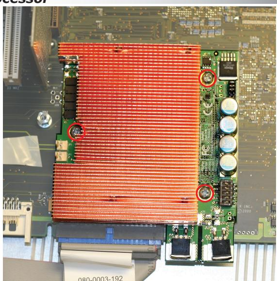
Remove the beige cap from the bottom of the upgrade card. Align the 3 circled screw holes, and gently but firmly press the upgrade card down onto the logic board. Insert the screws you removed from the original processor card.
