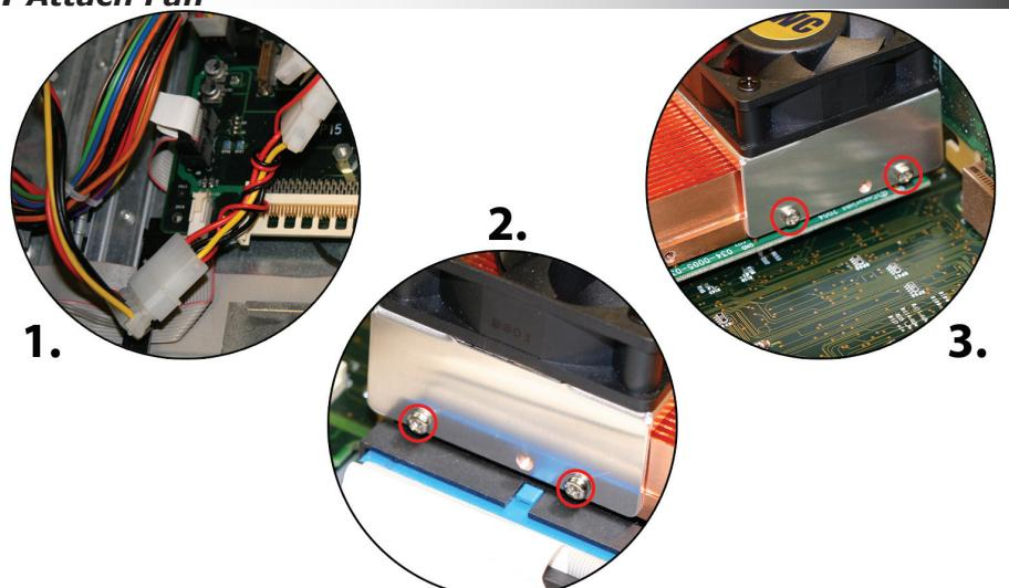
Plug the fan connector jumper onto a spare hard drive power plug. Insert the 4 included small Phillips screws through the holes in the fan assembly and attach to the heatsink in the location shown. You may need to remove the video card to insert the screws more easily. Some systems do not have enough clearance to screw in the screws - 2 will hold the assembly without issue.
