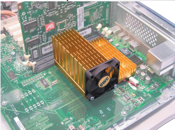
Installation of the processor daughter card is the same on all systems, simply align the 3 screw holes in the card and gently place over the logic board. Gently but firmly press straight down on the two rearmost screwholes until you feel the card "click" into place. Insert the included screwdriver and tighten the encapsulated 3 Phillips screws into the 3 screw holes. You're all done - **Enjoy your new processor!**
