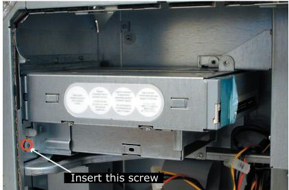
Insert the two Phillips screws you removed from the optical drive carrier.
