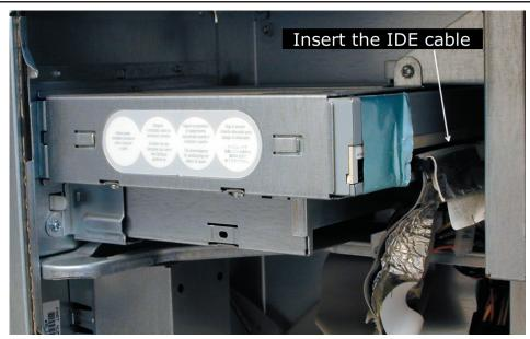
Replace the IDE cable you removed from the back of the optical drive. If you have a ZIP drive installed, you will need to replace that IDE cable as well (not shown).
