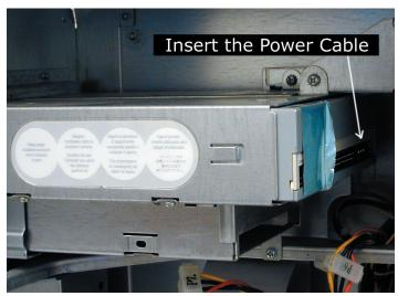
Replace the power cable you removed from the back of the optical drive. If you have a ZIP drive installed, you will need to replace that power cable as well (not shown).
