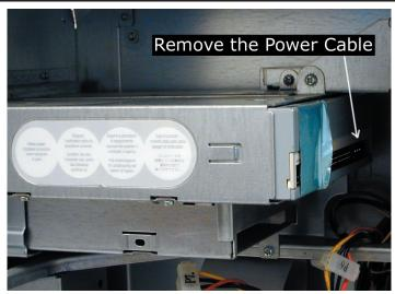
Reach in and gently remove the power cable from the back of your existing CD drive (and, if installed, your ZIP drive, not pictured). Lay them forward, out of the way, as shown.
