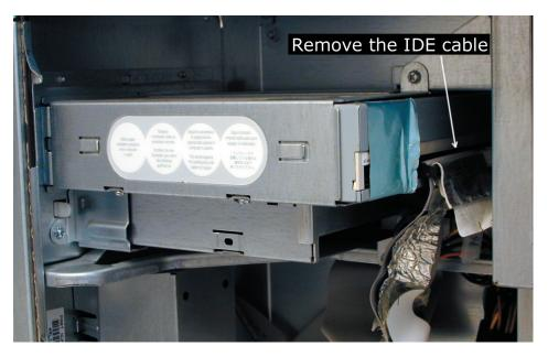
Begin by opening your system and touching a metal component such as the CD-ROM bay to ground yourself. Always be aware of static while working in your system, you can use a grounding wrist strap if you wish. Reach in and unplug the IDE cable from the back of the optical drive you are removing. If you have a ZIP drive installed, you will want to remove the IDE cable from it as well (not installed, and not pictured).
