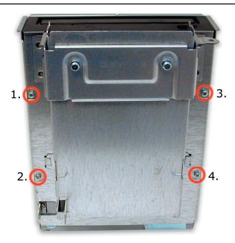
Insert the 4 screws shown here from the bottom of the CD drive carrier and you're ready to reinstall the new optical drive.
