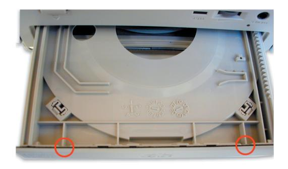
Press in with a screwdriver to unlock release tabs to slide the front drive door off of the drive tray.
