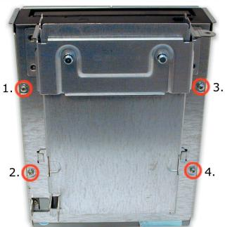
Remove 4 screws from bottom of drive
