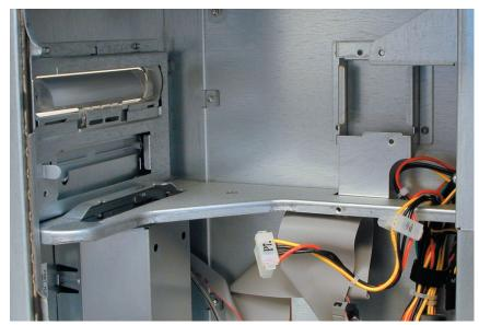
Once the two screws are removed, the CD drive bay will slide rearward and toward you, out of the computer.
