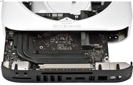
Slide the logic board out of the chassis carefully. Keep it as flat as possible to avoid interference with the memory slots.
