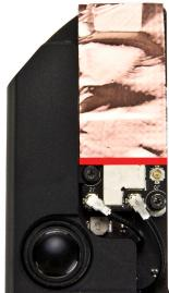
Remove the paper backing from the EMI shielding material provided in your OWC Bluetooth shielding kit. This will allow the shielding material to stick to the Airport/Bluetooth card. Apply the shielding material to the Airport/Bluetooth card as shown above, making sure to keep the material above the line in the picture. This will leave room for the Airport antenna to be plugged into the card later (step 11)
