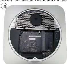
Gently lift up on the Airport antenna cover from the side closest to the logic board.
