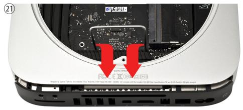
Carefully push down and pull back on the tool until the I/O wall separates from the housing slightly.
