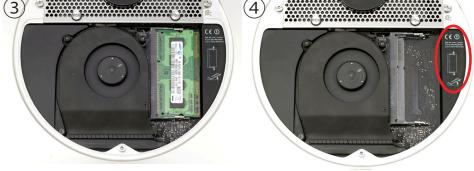
Remove the 2 SO-DIMMs from your Mac mini. Instructions to remove and insert them are inside the bottom cover on the right side next to the SO-DIMM slots.
