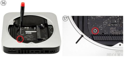
Remove the long Torx T6 screw from the chassis. It goes through the logic board and into the top cover.
