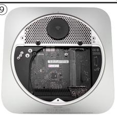
Using the Torx T8 screwdriver, remove the 3 2mm hex head (the Torx is the same size as a 2mm or 5/64 hex bit) screws that are used to hold the bottom cover onto the Mac mini. Do not exert too much force, Torx drivers are not as strong and can strip if you are not careful. Also remove the 2 Torx T8 screws opposite the Airport antenna. These secure the bottom hard drive in place.
