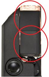
Apply the two original EMI shielding stickers back onto the Airport/ Bluetooth card on top of the newly applied shielding material. As shown in the picture, the sticker with the flap should be placed at the bottom, with the flap facing to the right.
