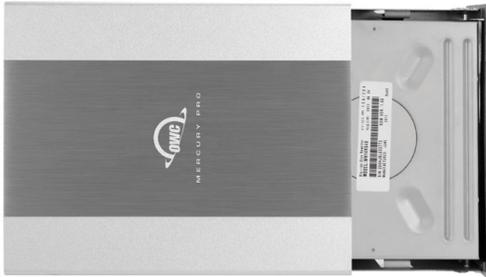
6. Once all eight screws are affixed, slide the inner chassis back into the outer enclosure until the front bezel contacts the outer enclosure.
