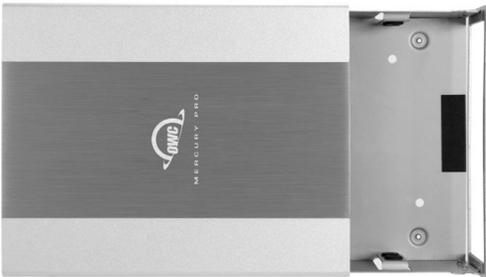
3. Push on the rear cover plate in order to slide the inner chassis out of the outer enclosure, as shown at right. Do not grasp the inner chassis by the front bezel, as it may bend slightly. Remove the screw packet and set it aside.
