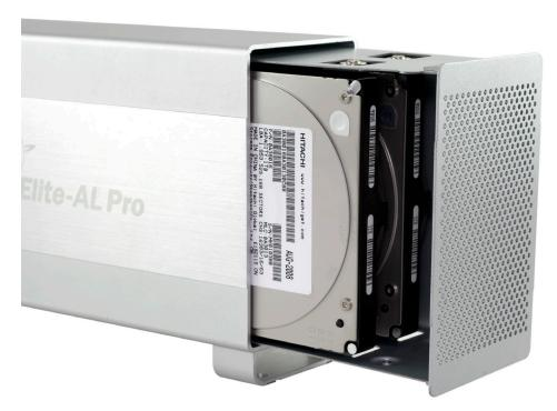
Slide the assembled chassis back into the enclosure from the front to the rear.
