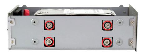
Secure the 2 hard drives into the chassis by inserting the 8 Phillips screws (4 each side) through the black rubber anti-vibration grommets, and into the hard drives. You may have to lift up a bit on the drives to get them into position. Firmly tighten the 8 screws to secure your hard drives into the chassis.
