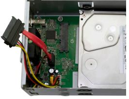
drive position, and connect one of the red SATA cables to the hard drive you are installing in the lower position, and place the hard drive into the chassis.
