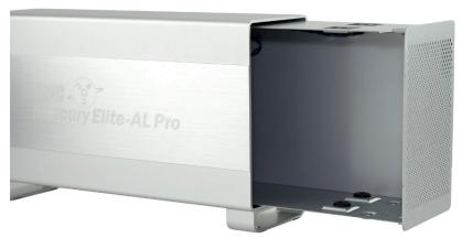
From the rear of the enclosure, push forwards on the interior to slide the chassis out of the outer shell.
