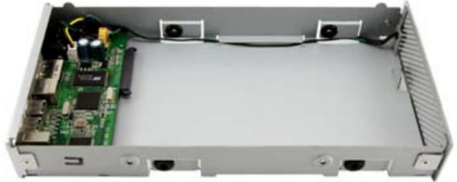
Here you see the OWC Mercury Elite-AL internal drive tray compartment. Insert your SATA 3.5" hard drive in the bay, and fully seat the drive connector onto the bridge board. The bridge board is the green circuit board pictured to the left in this photograph. You will see there is a connector built onto the bridge board that will interface with the drive, providing power and signal connections - no cables to connect!
