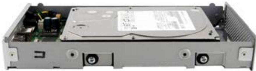
On the sides of the hard drive bay you will see 2 black rubber mounting grommets. You should see the holes in the side of your hard drive through these black rubber grommets, insert the provided screws through the rubber grommets to secure the hard drive inside the drive bay. These rubber grommets will help dampen noise and vibration, and also shock protect the drive. Repeat on the other side of the drive enclosure.
