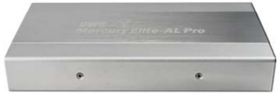
On the bottom of the OWC Mercury Elite-AL enclosure you will find 2 Phillips screws. Remove those two screws and the drive compartment will slide out towards the front of the enclosure. Remove the outer shell to proceed with drive installation.
