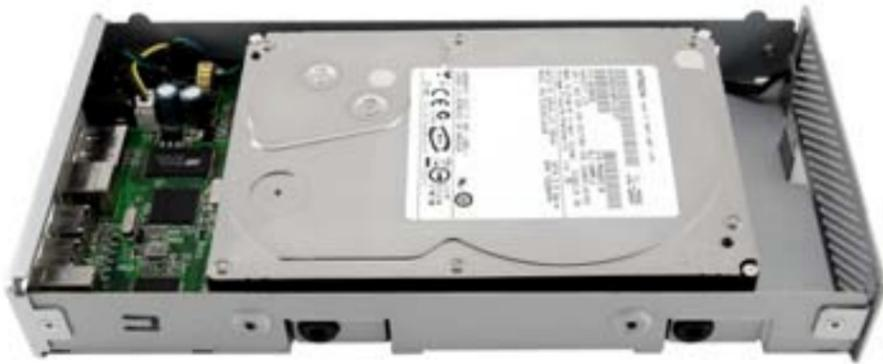
Here you see the hard drive fully inserted into the enclosure. Once you have inserted the drive, proceed to the next step, attaching the hard drive into the drive bay.
