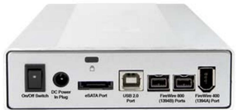
Now that you have your hard drive assembled, take a few moments and look at the back of the OWC Mercury Elite-AL Pro drive enclosure. Depending on the model purchased, you will see there are a multitude of interfaces that the drive enclosure supports. From the basic FireWire 400 / USB 2.0 enclosure, to the 'Quad Interface' model pictured here, the OWC Mercury Elite-AL Pro supports most any computer.
