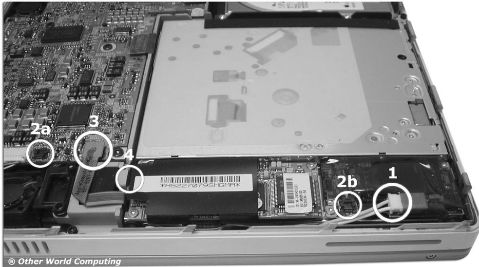
Start by attaching the drive controller cable on the back of the drive to the logic board. If there was a yellow piece of Kapton tape when you removed that cable, reattach it now.
