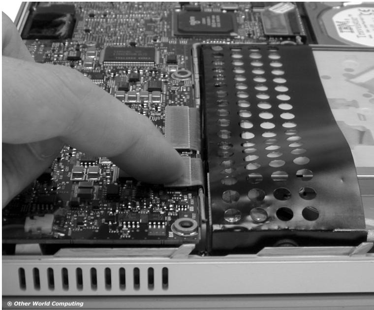
Once your new OWC Mercury Optical drive is inserted fully into the CD bay, insert the controlling cable onto the connector on the logic board. Be sure that the cable is fully lined up, it does take a bit of adjustment so it will seat into the connector fully. If your system had yellow tape covering the two connectors, reattach it now.
