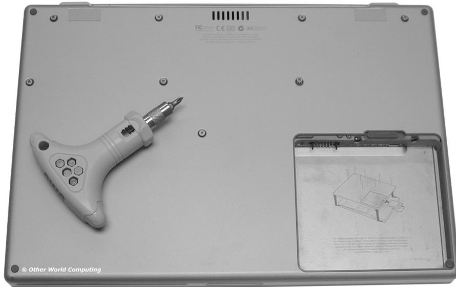
Place the bottom back onto your PowerBook and line up all of the screw holes. We recommend partially inserting each screw only enough to line the hole up, and proceeding to the next screw. Frequently PowerBooks will have a screw or two that are extremely difficult to get seated fully, if you encounter resistance while inserting the screws, you can usually press the case bottom back toward the rear a bit more and alleviate the pressure on the screw, allowing it to be tightened for a snug fit.
