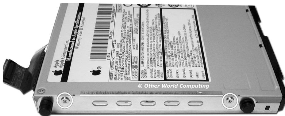
Turn the drive around and remove the two Phillips screws that attach the small left frame to the drive. Set all parts aside in a safe place.
