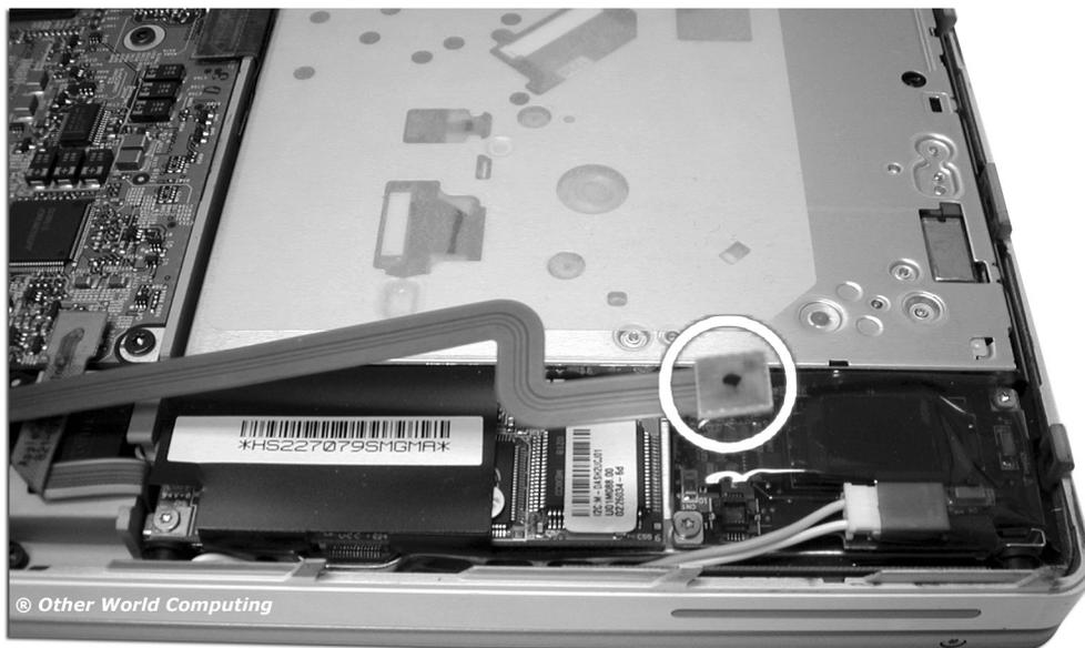
Begin removing the drive by gently lifting up on the ribbon cable attached to the inverter board, circled here.
