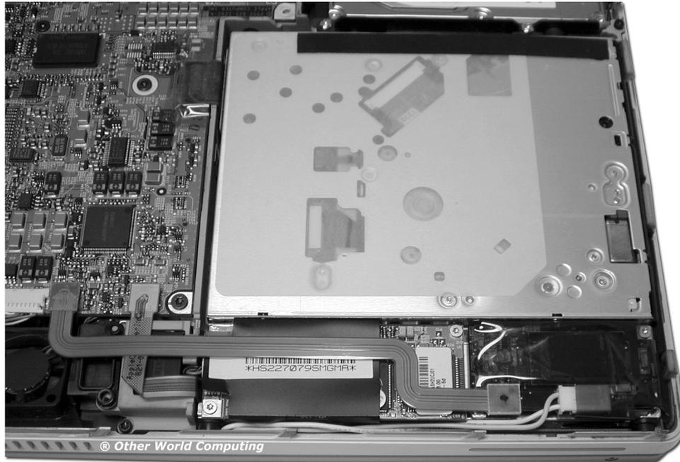
Upon removing the bottom shell of the PowerBook, you will see the optical drive on the left side of the computer. Turn the machine so the drive is oriented facing you, as shown in this picture. There are a number of cables and connectors you need to unhook to remove this drive. The cards attached to the drive brackets are a modem (left) and the inverter board for the display (right).
