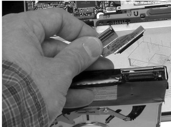
Another picture of the cable being removed, showing the connector in more detail.
