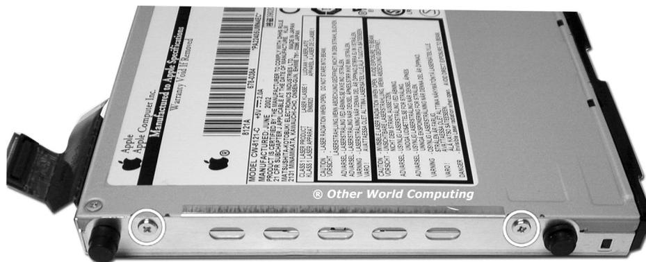
Reattach the small bracket to the left side of the drive using the Phillips screws you removed from it. The old drive is shown in this picture, installation is identical.
