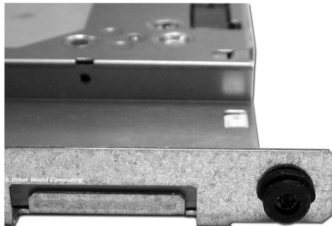
**Rubber Grommet is half-moon shaped. Put the cutout area to the bottom of the drive.**
