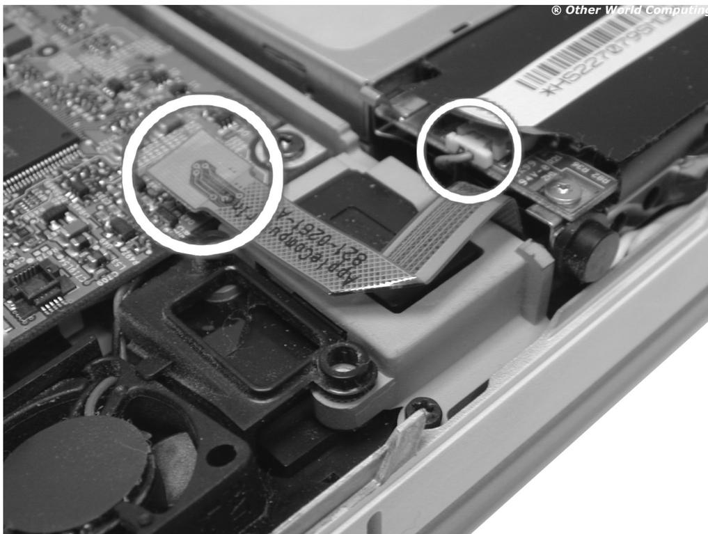
Look back at the outside of the drive assembly and you will see two more connectors that need to be detached. Unplug the ribbon cable from the logic board (it goes to the modem, underneath the drive), and also the 2 wire cable from under the edge of the black plastic cover on the modem card. That cable will need to be pulled straight out of it's connector toward the back of the PowerBook.
