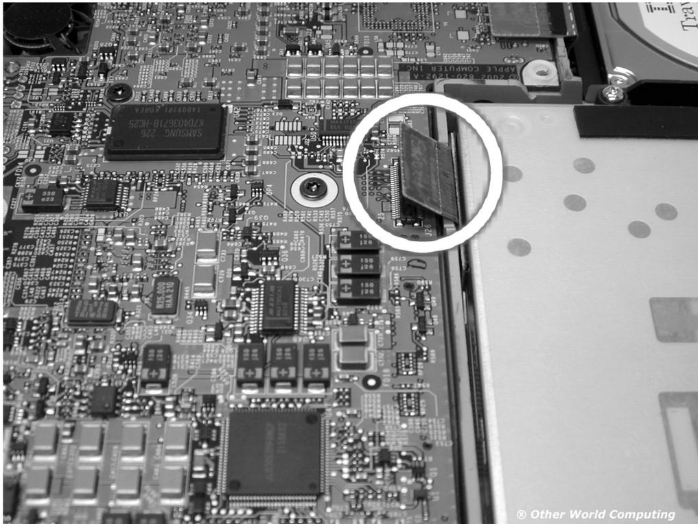
At the top of the drive you will see a flat ribbon cable attached to the main logic board, it may be covered by a yellow piece of kapton tape. If it is, remove the tape gently (you will reuse it), and lift up on the ribbon cable from the logic board side gently, as shown.
