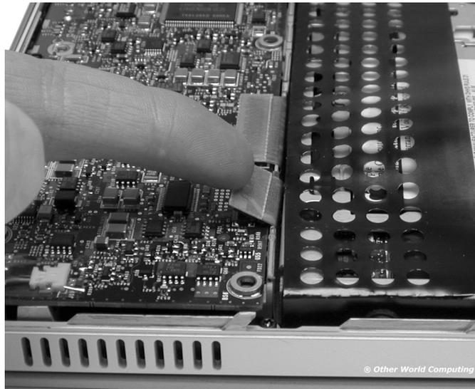
Begin removing the CD-ROM drive by detaching the cable that controls it from the main logic board as shown. You may find a yellow piece of tape covering the cable you need to remove, gently peel it off of the logic board, you can reattach it once the installation is complete. Your fingernail is probably the best choice to remove this cable from the logic board, you only need lift it up enough to dislodge it from the connector.
