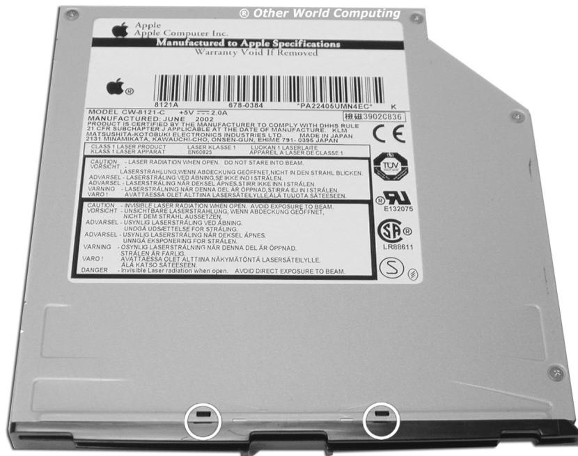
Turn the original drive on it's back and point the slot toward you as shown in this picture. Using a small thin straight screwdriver, or a paperclip, press gently on these two release tabs circled in this picture. You will find two more tabs on the bottom side of the drive (pictured below), and also one on the side. Once you release the tabs, you will see the other capture points and the removal is simple. Be patient, and do not break the tabs.
