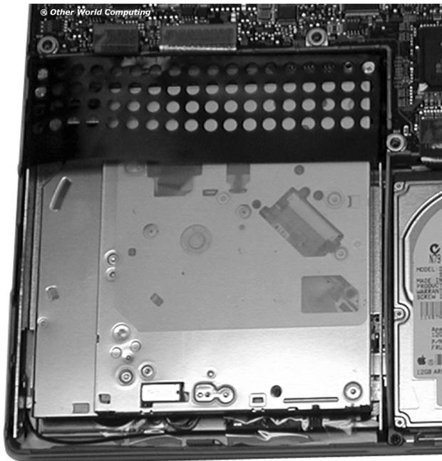
Your new OWC Mercury Optical drive should fit snugly into the drive bay. Run your fingers along the perimeter of the drive to be sure that it fully seated into the bay, it should not protrude from the left side at all, the half-moon grommets will settle down onto the posts that align the height perfectly.
