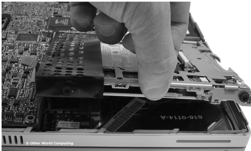
Set the new drive into the bay (old drive is pictured, but the fit is the same). **NOTE:** The label side of the drive will be **DOWN**, reversed from what the original drive was. Be certain when you have the holes on the right side of the bay lined up and pivot the new drive down into the bay that you have the controlling cable flush with the rear of the drive, otherwise it will catch and impede your movement of the drive downward.
