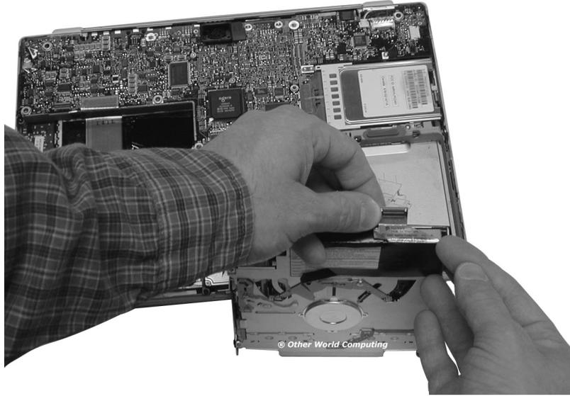
Take the CD-ROM drive and turn it so you can see the cable attached to the back of it. Gently use your fingernails to rock the cable gently, removing it from the connector. Set the cable aside.
