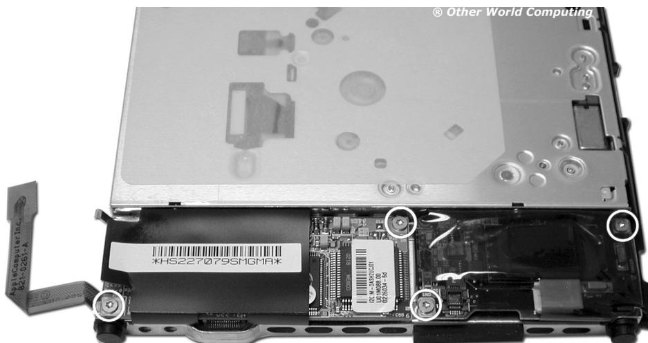
Reattach the 4 Torx T-6 screws you removed from the boards back onto the assembly, securing the cards in place.
