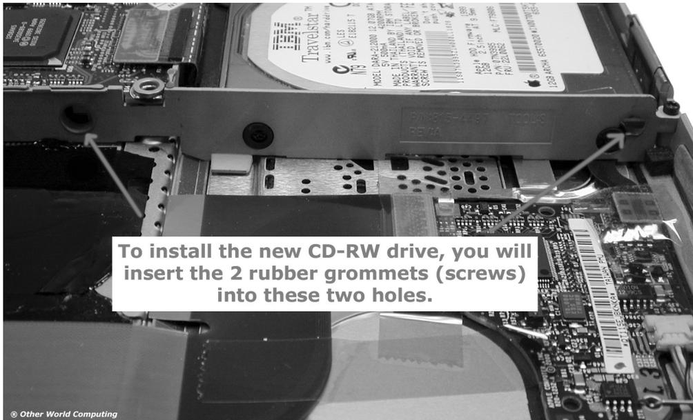
Now that you have the OWC Mercury Optical drive prepared to reinstall into the PowerBook, take a moment and look inside of the CD-ROM bay where the new drive will be placed. Note the two holes that are highlighted in this photograph. The grommet and washer will be placed into these holes when you install the new drive. Note that the rear hole is deeper than the front, as the front will not protrude into the hard drive bay when installed.
