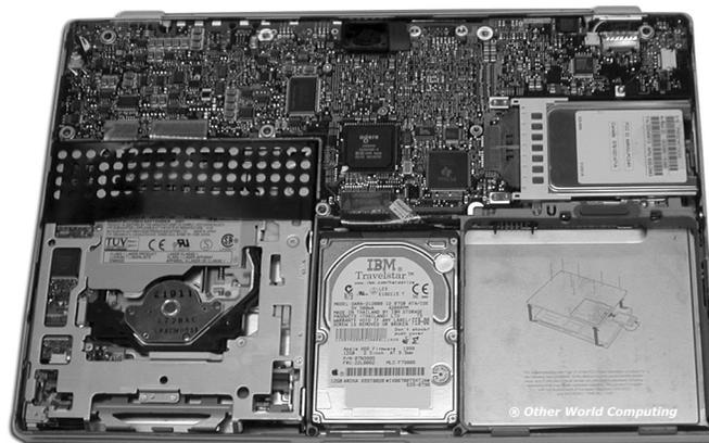
Gently remove the bottom of the PowerBook and expose the logic board / HD / CD Drive. Note on the bottom left is the object of this upgrade, the CD-ROM drive. You may want to take a few moments and remove any dust or lint that has become trapped inside of the computer, especially at the top center, the cooling fan.
