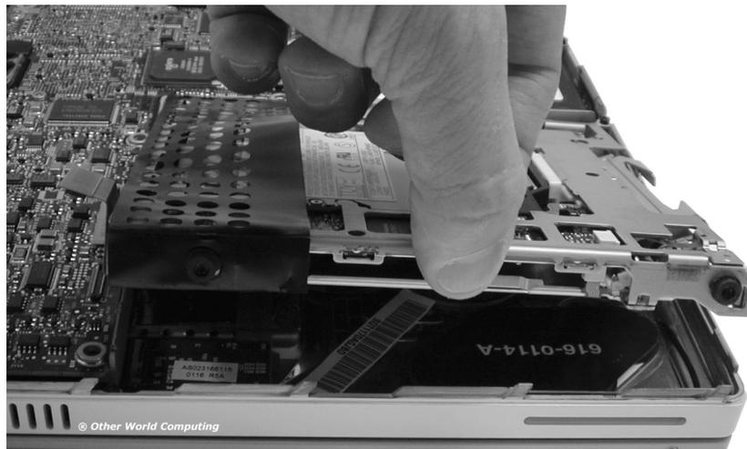
Once the cable has been unhooked, you can then grasp the side of the CD-ROM drive as shown and gently lift it out of the computer. You're lifting on the side of the drive, not the front. Notice the 2 screws and rubber grommets attached to the CD-ROM drive, they aren't captive held into the frame of the computer, they are held in by compression once the bottom is attached to the computer.
