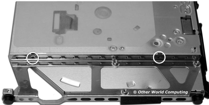
Remove the two Phillips screws from the large right metal frame. Notice that the screw on the left in this picture is a zero draft head - very flat, and it will need to be put back into this hole, otherwise the modem card will not fit flush back into place upon reassembly. Set the frame aside.
