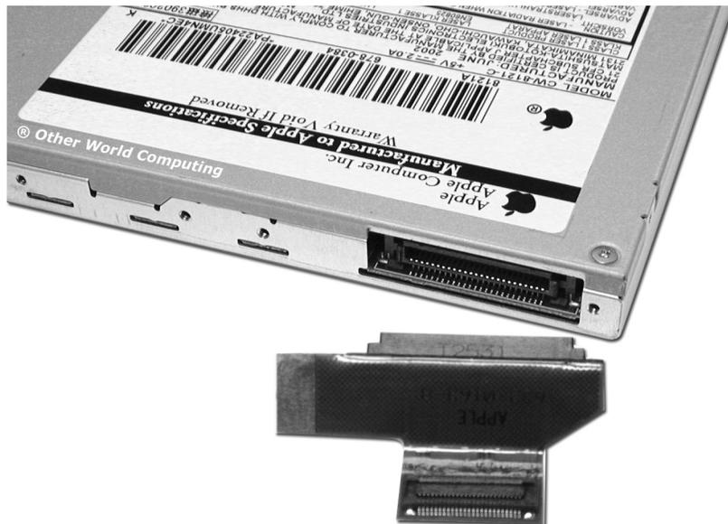
Remove the drive connector cable from the back of the drive and set it aside.
