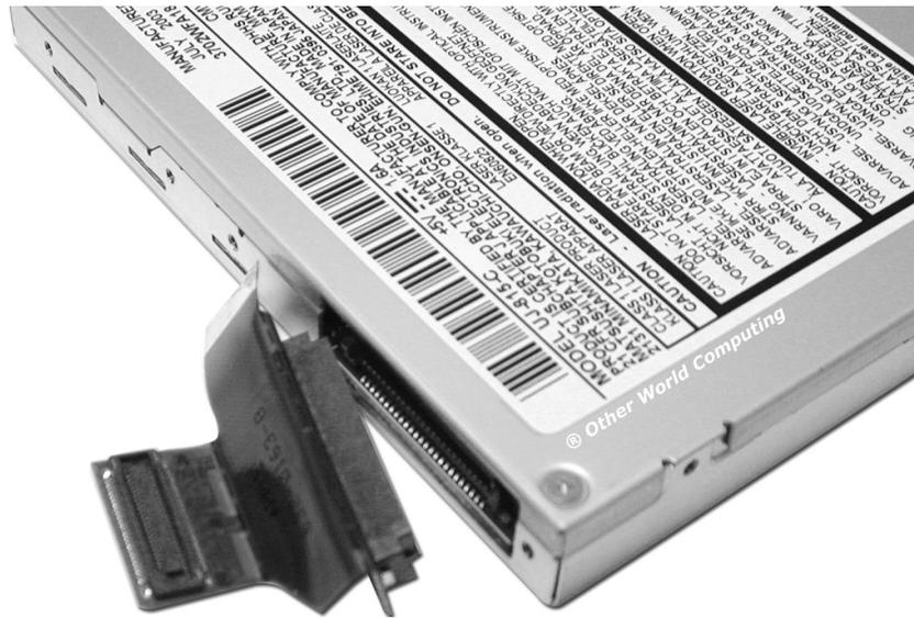
Attach the drive controller cable to the back of the new drive as shown. It will fit flush once in place.
