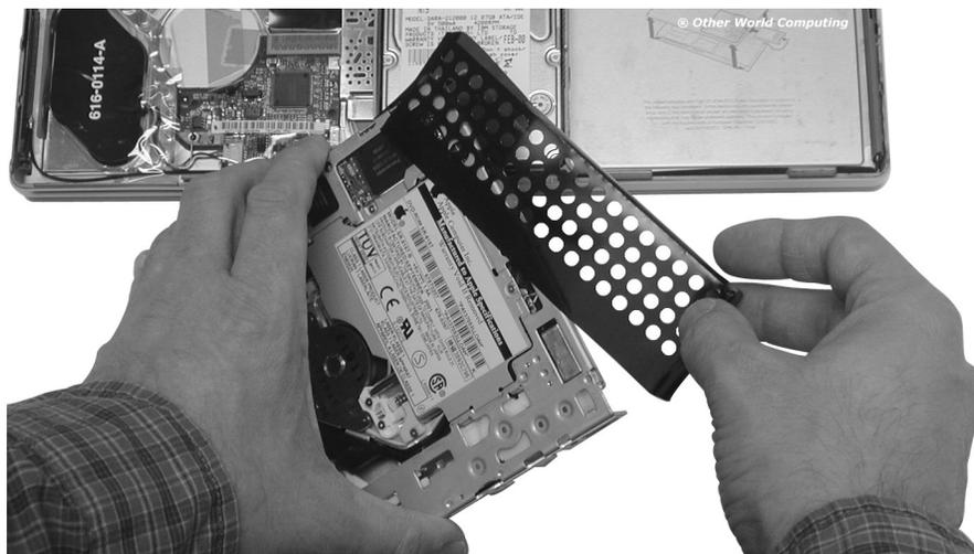
Once the screws have been removed, slide the thin plastic drive shield off of the CD-ROM mechanism. If you had to tear any part of it to remove because of it being stuck inside of the machine, take a moment and examine where it was torn and use a bit of tape to repair it.
