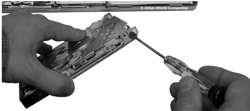
Insert the 4 Torx T-8 screws into the OWC Mercury Optical drive and place their grommets over the screw heads. Once again, the locations are:
