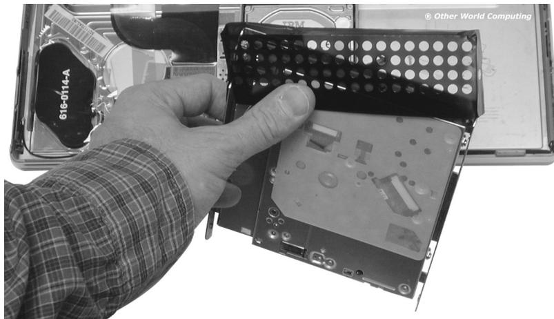
Slide the plastic drive shield over the rear of the new OWC Mercury Optical drive. This usually takes two hands to get it in place. The shield will fully cover the rear of the drive and the screw holes will be visible once you have it in place all the way.
