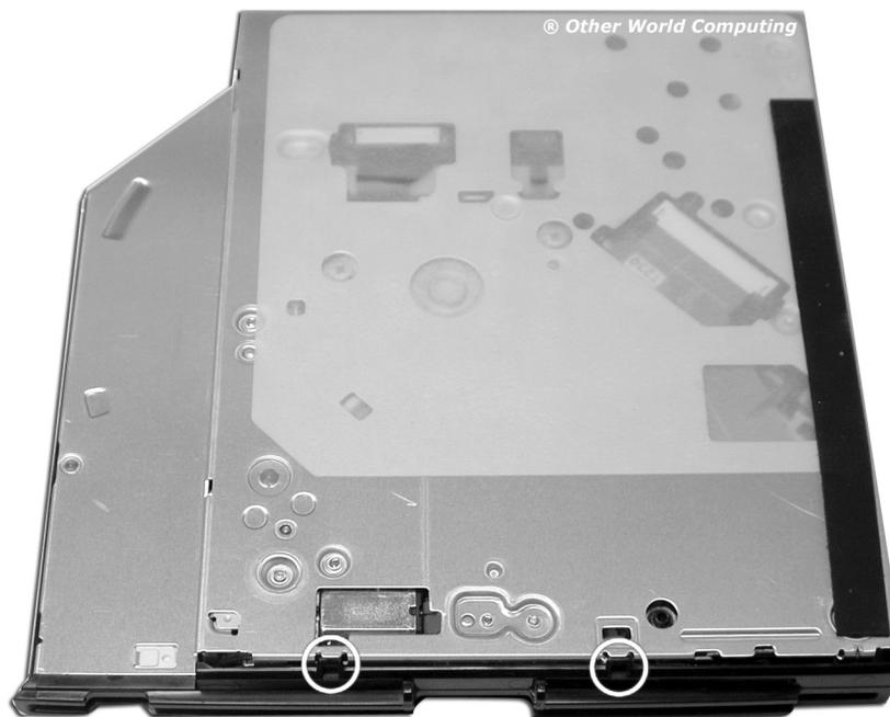
Remove and place the feed slot onto the new drive in the same way you removed it from the old drive, starting with the side tab and hinging the slot onto the drive mechanism, locking it into place.
