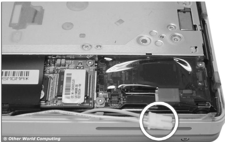
Unplug the white and pink cable from the inverter board by pulling gently straight back towards the modem, the cable is shown unplugged in this picture. The wires are very flexible silicone coated, do not pinch or cut them as they carry power to the LCD display.
