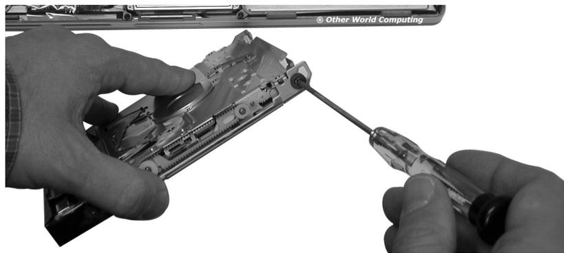
Use the Torx T-8 screwdriver to remove the 4 screws and grommets that are at the corners of the drive. You will notice that the screws are all identical, but there are 3 different types of grommets.
