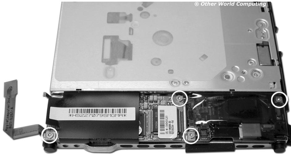
You are now ready to physically remove the drive from the PowerBook. Start by gently lifting up on the drive where the modem and inverter boards are at, angling the drive from the outside. The 2 rubber grommets that the drive rests on will allow the drive to lift freely on the outside, but not the inside. The inside grommets are captive and fit inside holes in the frame and you cannot lift from the middle of the computer.
