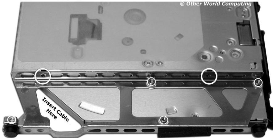
Begin assembling the new drive by placing the large right frame on the new drive. Attach the small zero draft screw on the left, and the regular screw on the right (circled with the large circles above). Gently slide the modem's ribbon cable through the slot shown above, placing the modem on the screw risers circled on the left. Do the same with the inverter board, placing it on the right, with the power connector toward the modem card.
