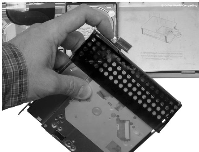
Align the cable you removed and fully seat it into the OWC Mercury Optical drive's connector. This will also help hold the plastic shield in place while you install the screws and grommets.
