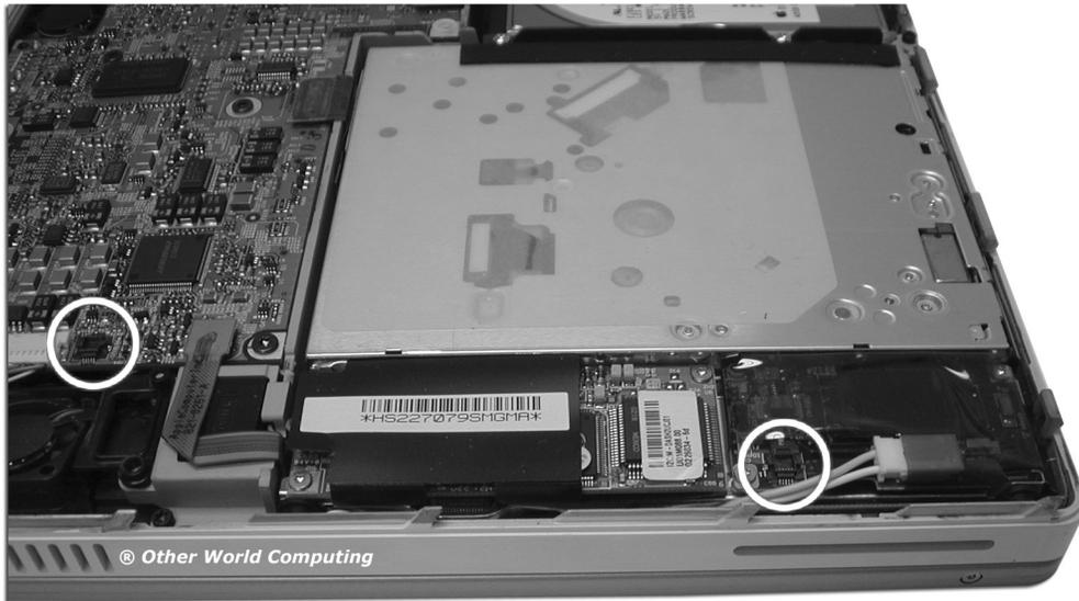
Detach the ribbon cable from the inverter board and then from the logic board - the two positions you remove the cable from are shown circled in this picture. Set the inverter ribbon cable aside.
