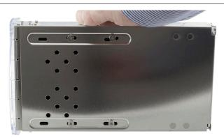
Turn the enclosure on it's side, removing the bottom plastic outer shell, and securing the drive you just placed into the enclosure with your fingers as shown above. Lift up on the hard drive mechanism and line the screwholes up with the cutouts on the bottom of the enclosure.
