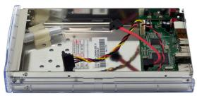
Remove the top cover from your OWC Mercury Elite Pro enclosure by sliding the top cover towards the rear of the unit. Then, remove the single Phillips screw securing the top metal shield, and lift up on it to remove, exposing the inside of the enclosure.
