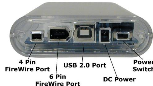
The power switch is 2 position. Left, towards the DC power port for ON and right for OFF. You must plug in either a 6 pin FireWire cable for bus power or the DC Power Adapter.
