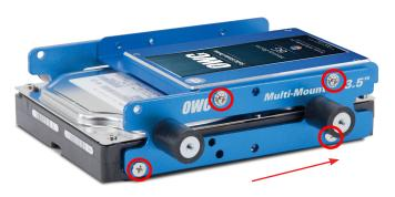
This is a completed assembly comprised of one set of 3.5" OWC Multi-Mount drive brackets, and one set of 2.5"-3.5" Adapter Bracket, all assembled into one unit. Be sure to orient the bracket so that the SATA ports both point towards the rear of the Multi-Mount.
