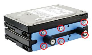
Once you have the right bracket installed, rotate the hard drive and attach the left side bracket using the same method.
