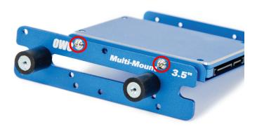
Once you have the 2.5"-3.5" Adapter Bracket attached to the 2.5" hard disk drive, you can install up to (2) 2.5" drives onto the 3.5" OWC Multi-Mount bracket.
