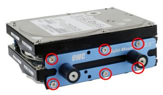
Begin by positioning the bottom 3.5" hard disk drive with the connection ports facing away from you, and then pick up the OWC Multi-Mount 3.5" drive bracket that has the white OWC Multi-Mount 3.5" silkscreening on it.
