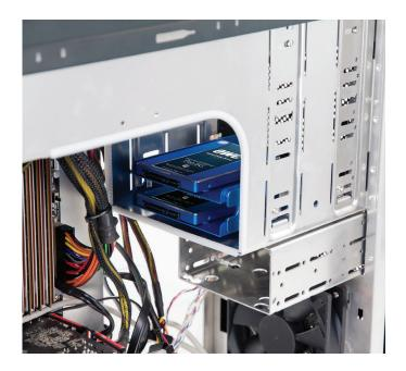
Here you see a PC case with the 2.5"-3.5" Adapter Bracket installed in a 5.25" (top) drive bay, But it also can be installed in a 3.5" drive bay (bottom).
