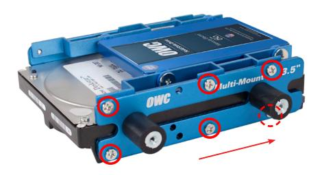
This is a completed assembly comprised of one set of 3.5" OWC Multi-Mount drive brackets, and one set of 2.5" OWC Multi-Mount, all assembled into one unit. Be sure to orient the bracket so that the SATA ports both point towards the rear of the Multi-Mount.
