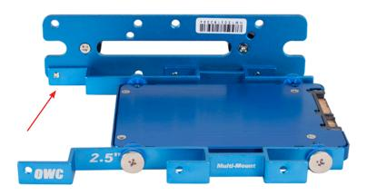
It is possible to install a total of two 2.5" drives onto the 3.5" OWC Multi-Mount bracket. Note the position of the bracket extension shown above (arrow) relative to the 3.5" bracket. This is important when creating a configuration with two 2.5" drives installed.
