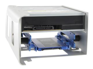
First, attach the completed Multi-Mount assembly to the optical drive cage using the four screws that Apple supplies (attached to the cage). Once the Multi-Mount is secured, start sliding the cage back into the optical bay, threading the large cutouts on the bottom of the cage with the large screws on the bottom of the bay.
