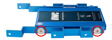
To install a 2.5" SATA drive into the Multi-Mount, place the 2.5" drive on the table in front of you, with the connection ports facing to the right side. Take the drive bracket and position it as shown above.
