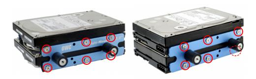
Begin by positioning the bottom 3.5" Hard Disk Drive (HDD) with the connection ports facing away from you, then pick up the drive bracket labeled as OWC Multi-Mount 3.5".
