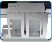
Grasp the optical bay with your fingers and pull straight out. The drive carrier may require a bit of shaking to dislodge it from its mounts. Disconnect the power and SATA cables from the back of the optical drive and set the carrier on a work surface in front of you.
