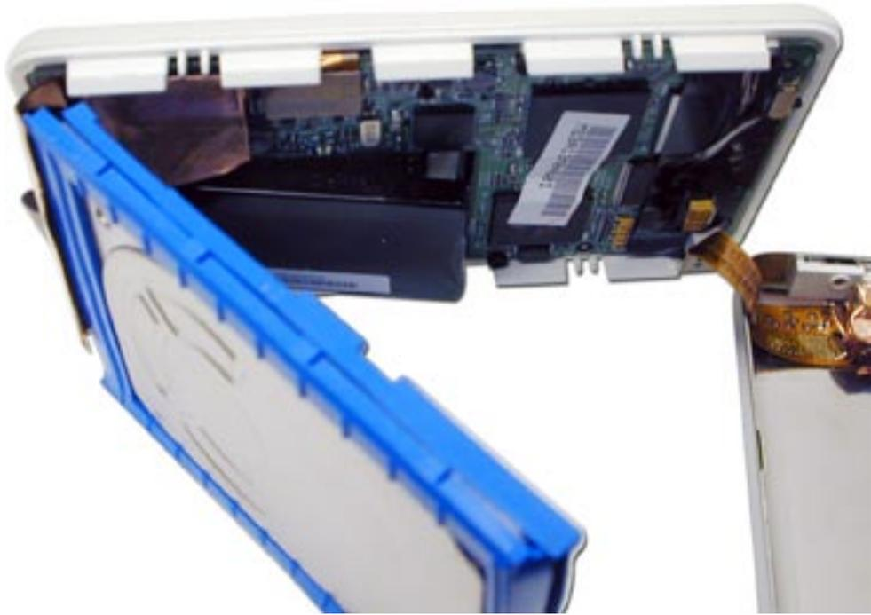
Lay the metal back cover flat on the work surface, and stand the iPod on it's edge as shown. You can gently lift the hard drive away from the inside of the iPod as shown, exposing it's connector on the logic board.
