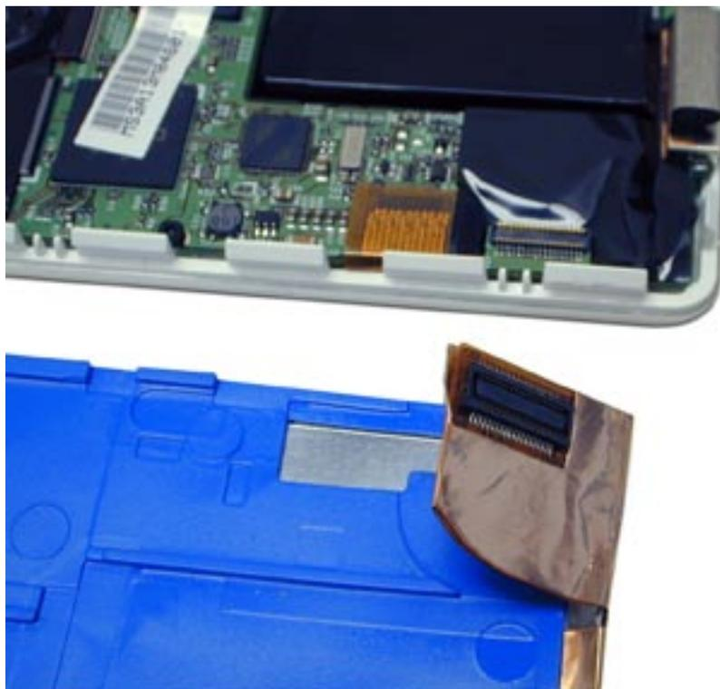
Detach the hard drive from the logic board using your fingernail or the nylon screwdriver tool, at the edge of the connector. Light pressure will release the connector from the board - set the hard drive aside.
