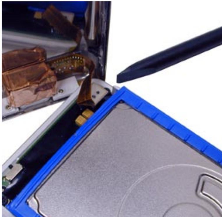
Another view of the ribbon connector, with the screwdriver tool pointing toward it. Do NOT remove the connector - it is not necessary to replace the battery.
