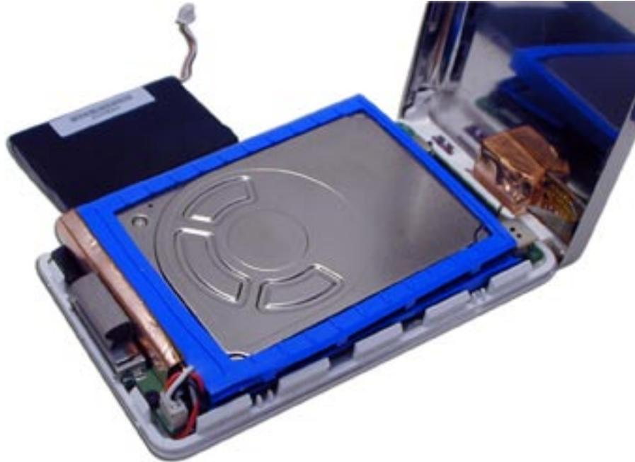
Set the hard drive back into the case and reattach the cable onto the logic board firmly. It may make a "click" as it's seated onto the logic board, that is normal, don't worry. You may find the attachment is performed more easily with the unit on it's side as you had it with the drive removal. Once complete, set the back cover onto the unit, being careful to make sure that the hold switch seats back over the internal switch properly.
