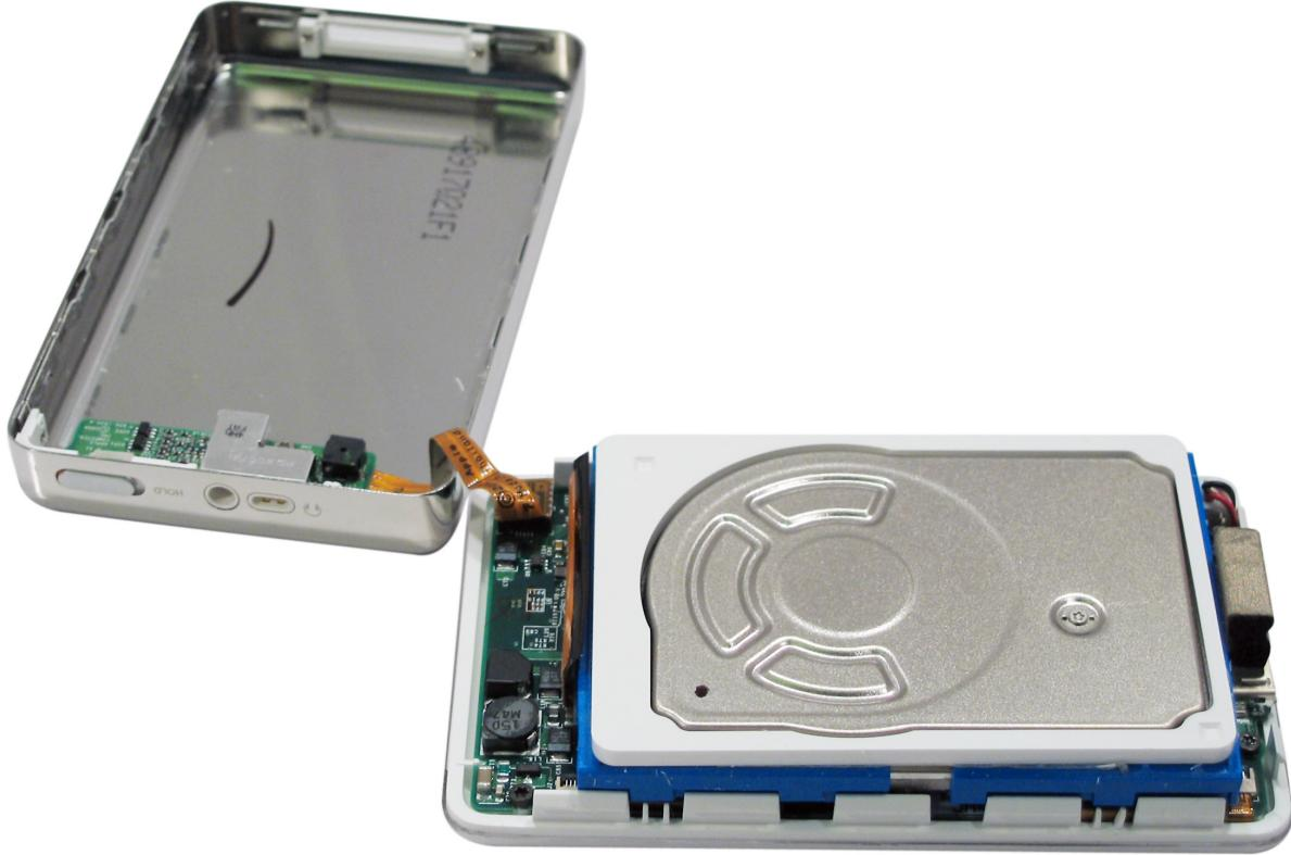
Place the back of the iPod back onto the front. Work from one side to the other, pressing the face onto the back. Use equal pressure around the perimeter of the iPod to close the case fully. Look at the dock connector when done, and make sure that the static shield is fully tucked in and the dock connector is not blocked.
