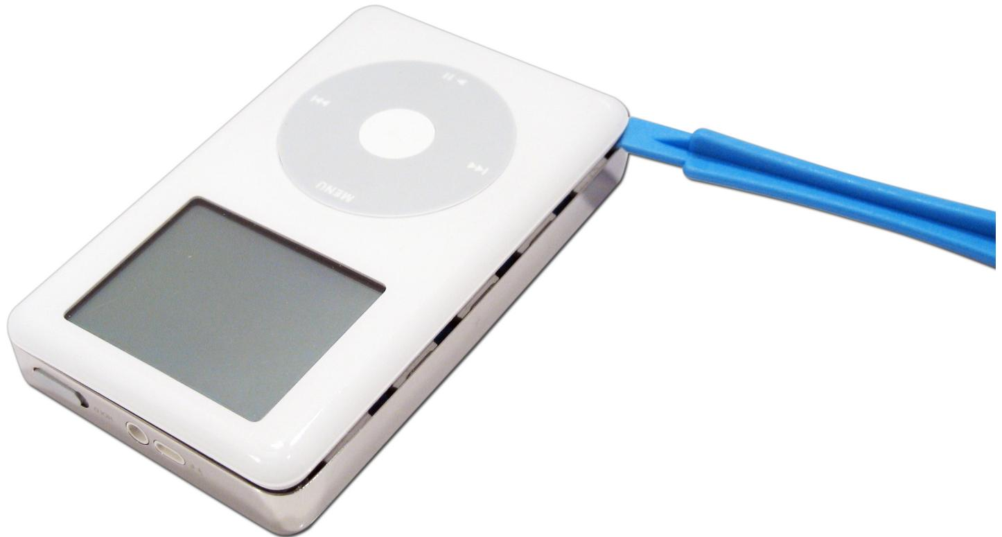
Once the tool is inserted, gently work it from the top edge to the bottom edge, releasing all of the clips on the left side. You may have to move the tool up and around the top edge to get that clip to release.
