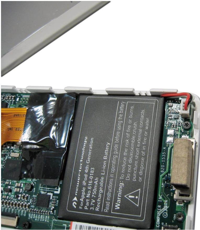
Insert the plug and route the wires as shown, over the top of the circuit board. Replace the 2 Torx screws that you removed previously.
