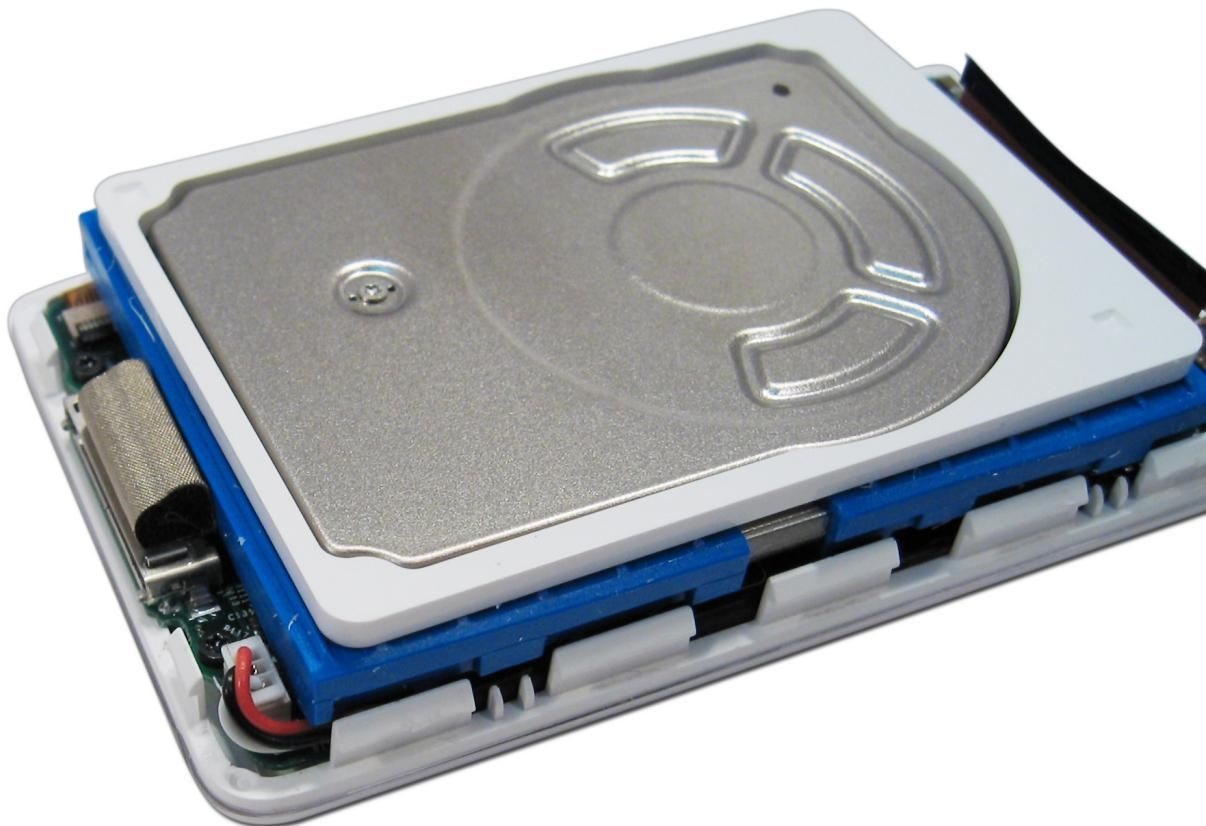
Place the hard drive back on the iPod, and line the connectors up. There is a plastic guide pin that will make sure you get the drive installed properly. Fully seat the cable into the hard drive, and then place it back on top of the iPod. Note the proper location of the new battery cable.
