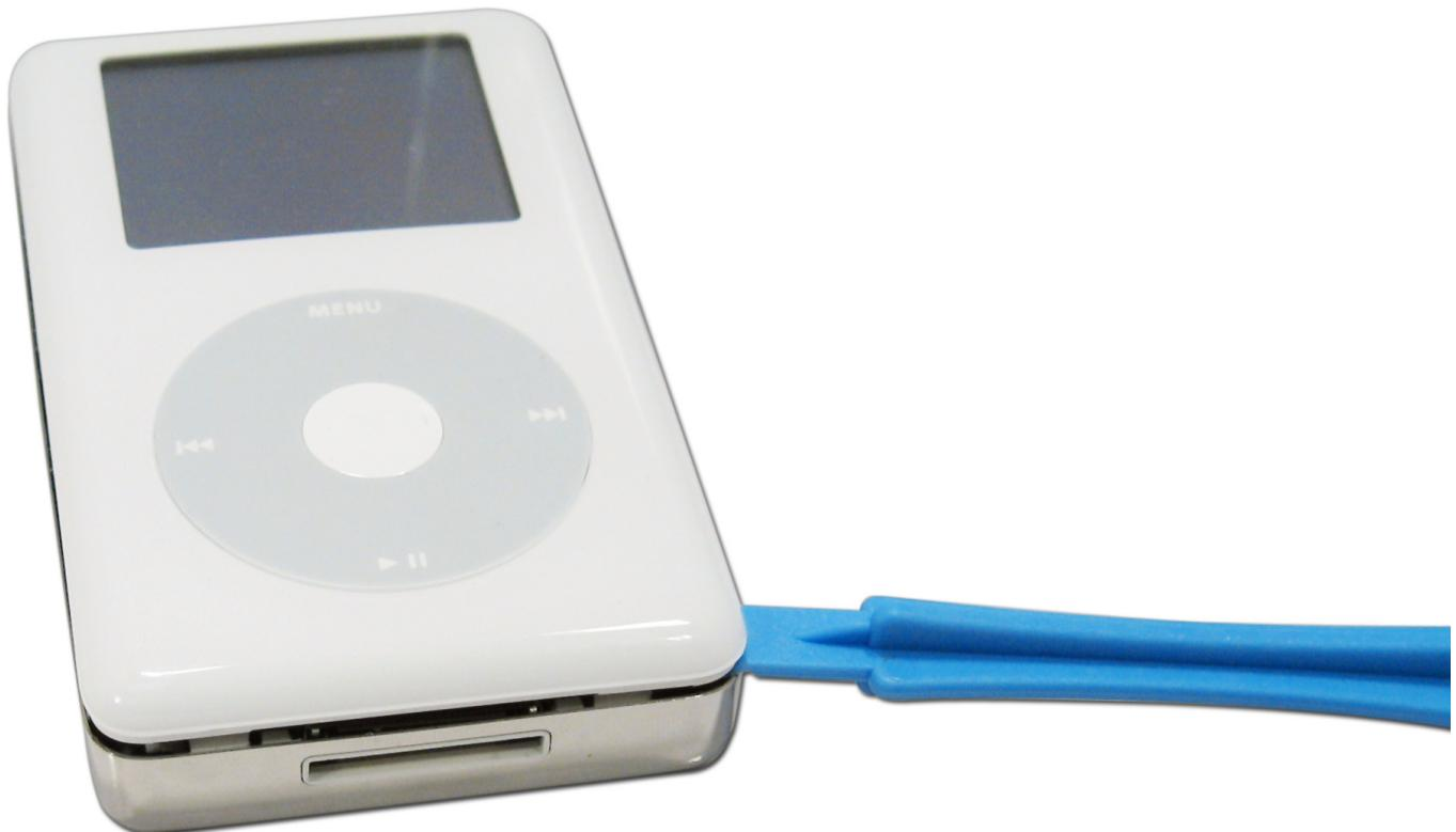
Work the tool around the bottom edge, and across the dock connector to the right side. Use extreme caution while sliding the tool across the dock connector, you can easily bend the metal around the dock connector as it is much thinner than the rest of the back shell. There are 2 clips, one on each side of the dock connector to release.
