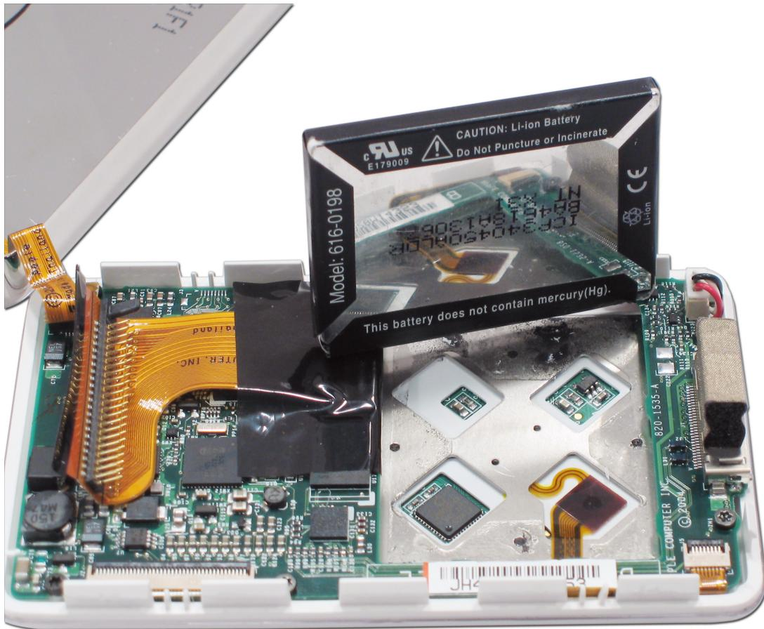
Here you can see the battery removed, and the "X" shaped pattern of adhesive under the battery.
