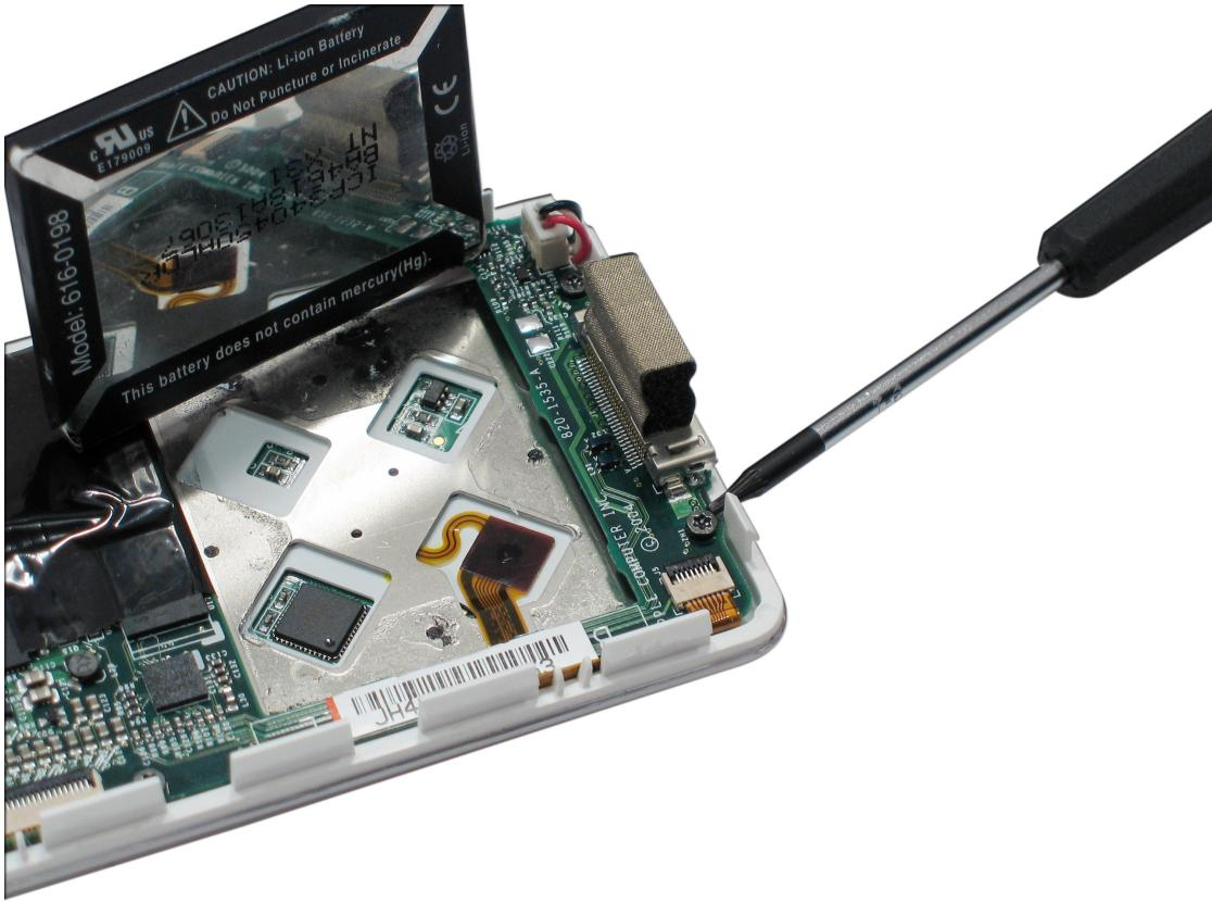
Once the battery is loose, you need to remove 2 Torx T-6 screws to lift the logic board up enough to remove the battery wire and connector. Remove the first screw shown here.
