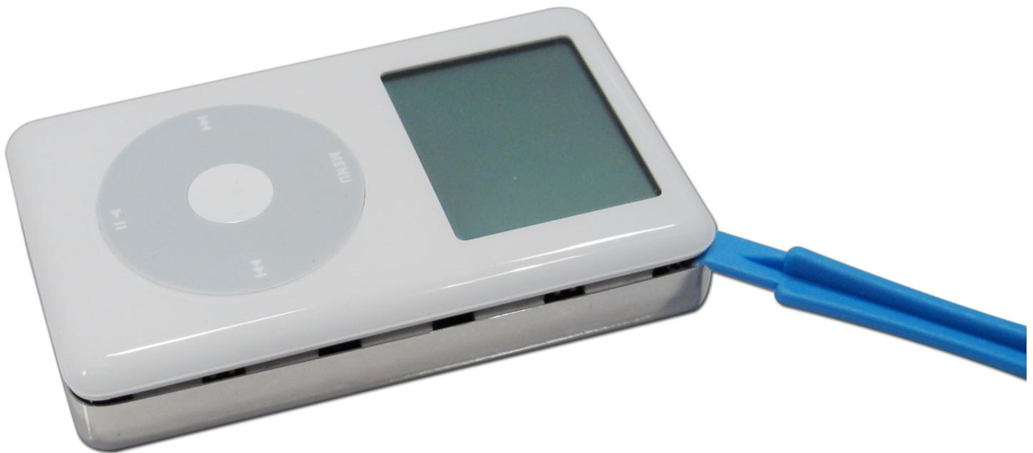
Finish releasing the back shell in the same manner as the left side, working the tool back and forth until the clips release. You once again may have to move the tool up and around to the top to get the shell to come off completely.
