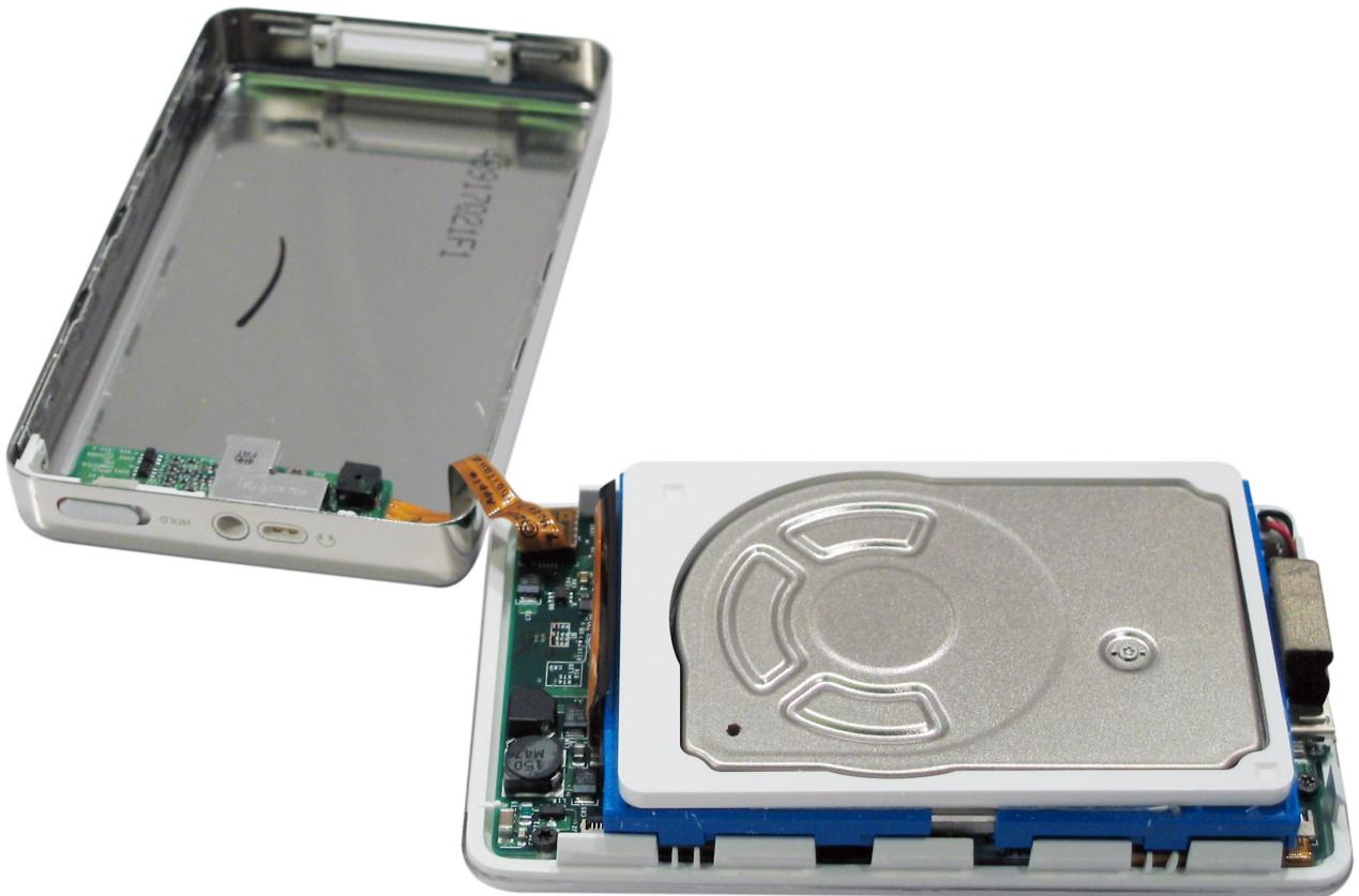
Once the back shell is released, place the iPod on it's face and GENTLY lift the back shell off, lifting up and away from the Dock connector. Do NOT place too much pressure on the cable that connects the back of the iPod to the front of the unit. Set the back on the work surface as shown.
