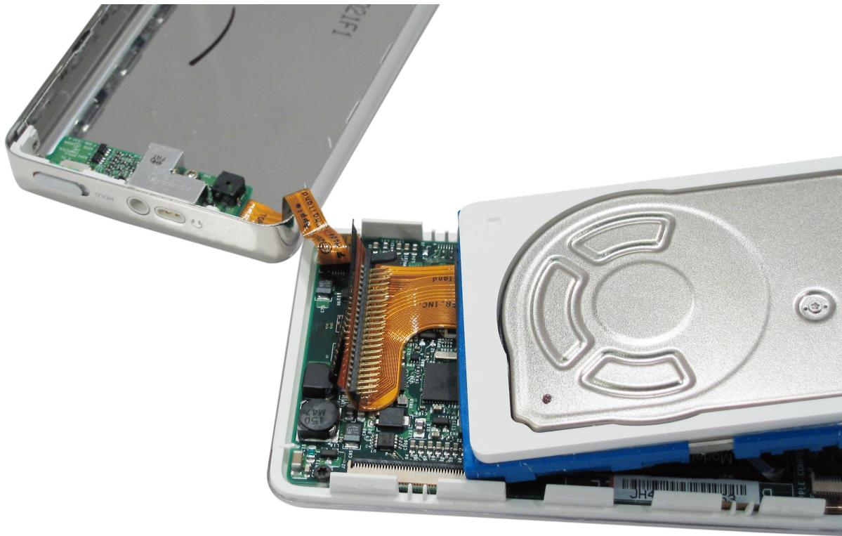
Lift up on the hard drive from the dock connector side about 1". On the opposite side, gently remove the connecting cable from the hard drive by pulling straight on the connector using the black portion of the ribbon cable, it's raised up above the drive a bit. Do not bend any pins on the hard drive while removing, use extreme caution. Once removed, place the hard drive aside.
