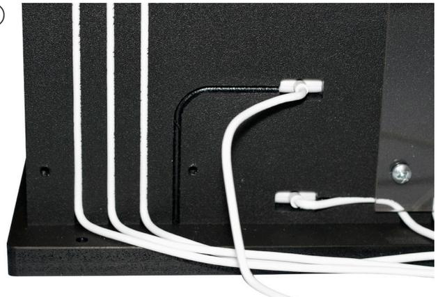
Once the plastic cover is removed, locate the dock cable that you wish to remove. From the bottom of the GripStand Station, lift up on the cable and remove it from the wire channel to release it.
