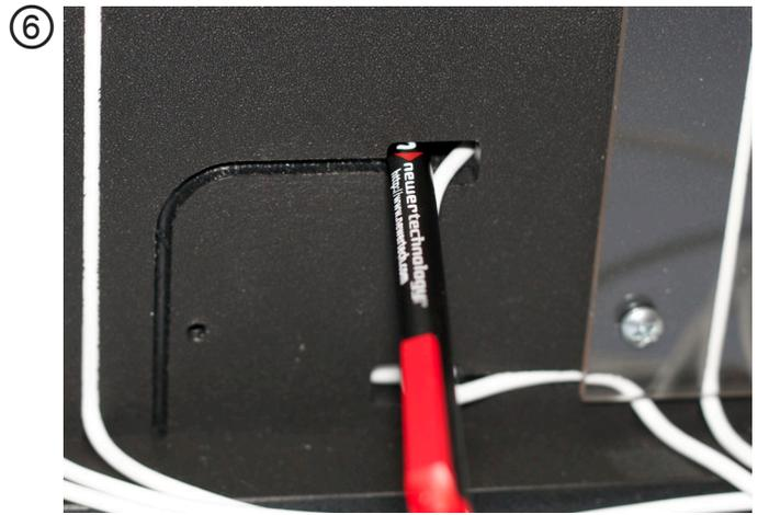
Using a retractable pen (a flat tool that you can push with, and not cut the cable is all that's required), gently push on each side of the dock connector to release it from the dock cable slot. Once you press it out of the slot, the pen will slide into the GripStand Station housing.
