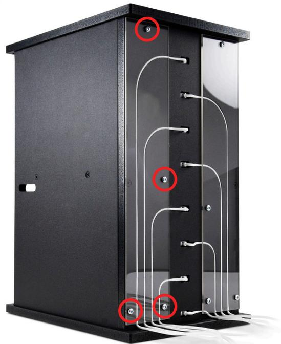
To remove a 30-pin dock cable, turn the GripStand Station so that you can see the rear and the dock cable channels. Determine which cable you want to remove (in this scenario, the second cable from the bottom will be replaced). Unscrew the four Phillips screws that secure the clear plastic cable cover (circled in red in step ②), and remove the plastic cover.
