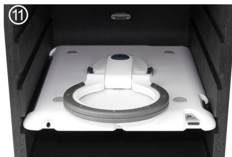
Make certain that the iPad is laying flat in the GripStand Station side guide rails and then firmly push in on the iPad, pressing the dock cable into the back wall of the GripStand Station. This seats the dock cable perfectly flat and straight into the retaining slot for the dock connector. Reinstall the cable into the guide channel and replace the plastic cable cover and the replace the black wire loom around the USB cables to complete the installation.
