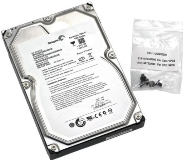
Make sure that the hard drive you wish to install (sold separately) is handy and remove the screws from the bag.
