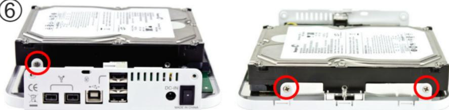
Insert the 3 large Phillips screws from the plastic bag into the drive enclosure securing the hard drive through the screwholes.
