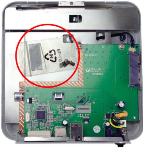
Untape the plastic bag with assembly screws from the inner chassis.
