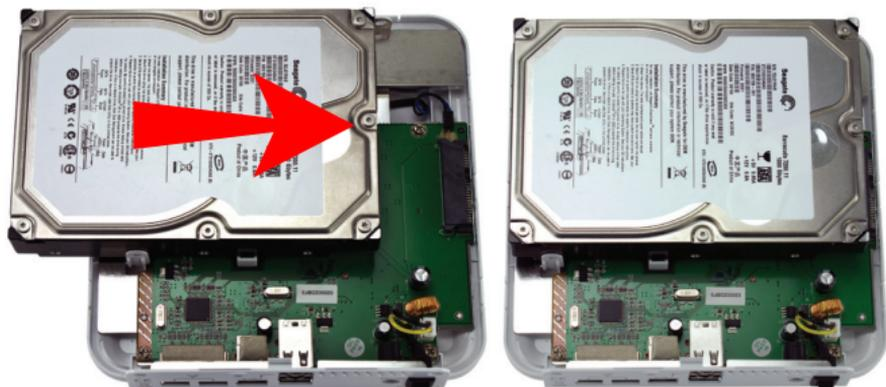
Place your drive into the chassis of the miniStack Classic. There are 2 mounting tabs with screwholes on the side furthest away from you in this photograph, and one screw post on the side closest to you.
