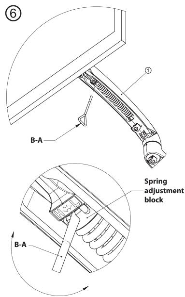
Adjust the tension on the NuMount Pivot VESA desk mount up or down to achieve the desired height and distance.
