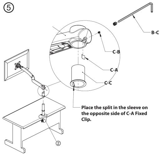
① Insert fixed clip (C-A) into the curved notch inside the NuMount Pivot arm.
