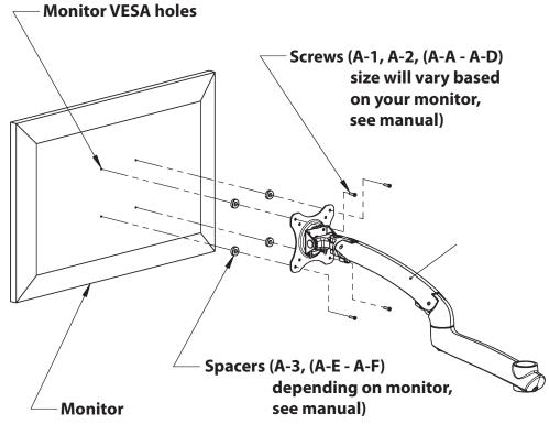
Attach your monitor to the NuMount Pivot VESA arm using the included screws and spacers. Check the manual for your monitor or computer to determine the correct size screws to use. There are screws and spacers included with this kit to accommodate most common possibilities.
