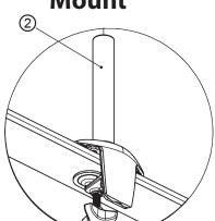
Fasten the desk clamp base onto your desk and secure tightly using the integrated knob. Make sure that the base is firmly pressed against the side of the desk work surface.
