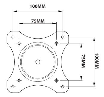
The NuMount Pivot VESA features mounting points for both 75MM and 100MM VESA compliant displays and computers.
