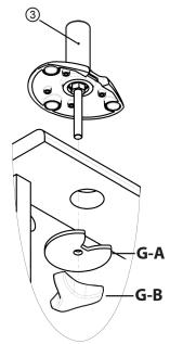
Optionally, the NuMound Pivot VESA desk mount includes a clamp for use in a desk grommet. If your desk has grommets in it, you can use this mount to secure the pivot arm. Clamp the desk grommet base to your work surface using the included mounting plate and wheel nut.
