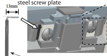
Insert white wire into slot on steel screw plate
