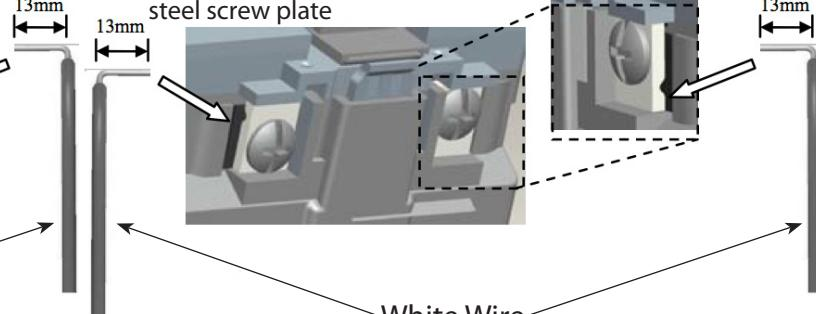
Insert bare or green wire into slot on steel screw plate
