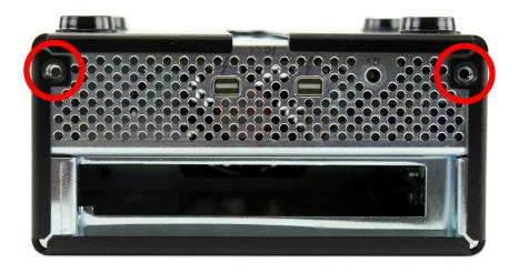
3. Remove the two Phillips PH2 screws from the bottom of Helios.
