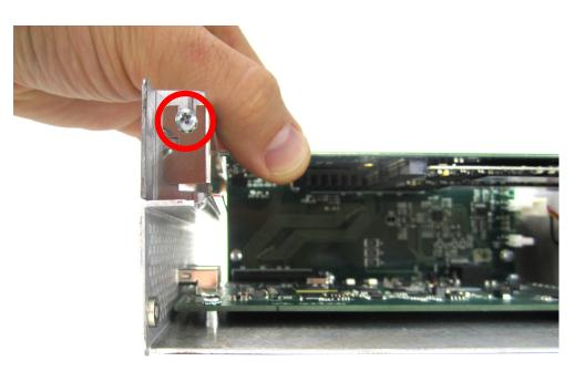
Carefully lift up the edge of the card until the bracket is stopped by the PCIe bracket screw, then fully tighten the PCIe bracket screw.
