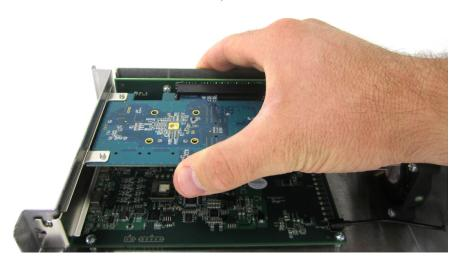
8. Replace the PCIe bracket screw. Do not fully tighten the screw.
