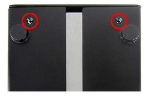
4. Turn Helios back over and place it on it's feet. Using your fingers, push the inner chassis out of the outer enclosure. Do not squeeze the sides of the enclosure while doing this.
