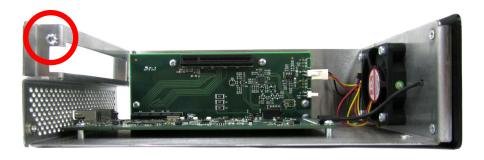
Remove the Phillips PH2 screw from the PCIe expansion slot. You are ready to install your PCIe card.
