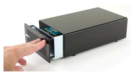
Align the screw holes and replace the bottom screws.
