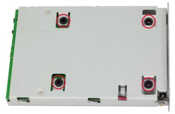
7. Using a Phillips screwdriver, insert the four included screws into the screw holes to fasten the drive to the inner chassis (shown below). When this is done, turn the inner chassis back over.
