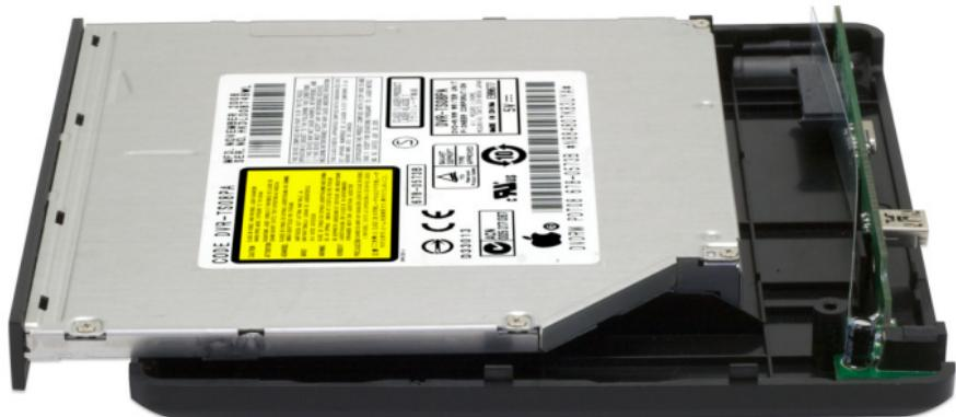
Remove the top cover of the enclosure by sliding it towards the rear - it will unlock and lift off.
