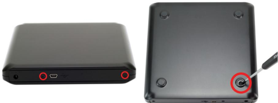
Place the top of the enclosure on the bottom, and sliding from the rear, lock it in place to the bottom of the enclosure.
